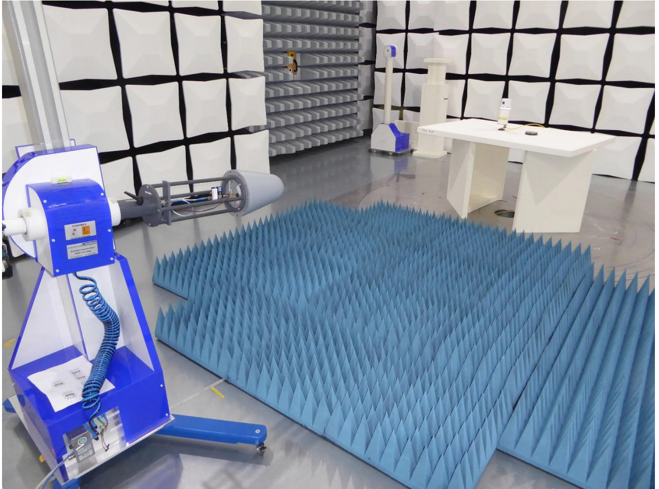
Test setup semi anechoic chamber TX spurious emissions from 1 GHz – 12GHz
