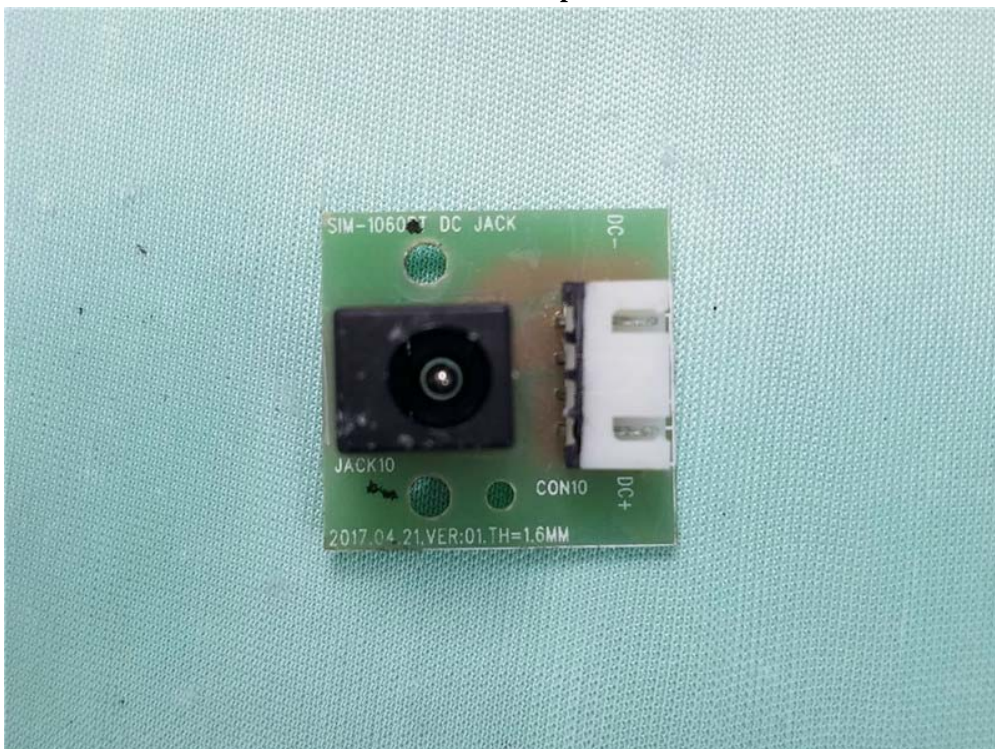
Inner Circuit Top View
