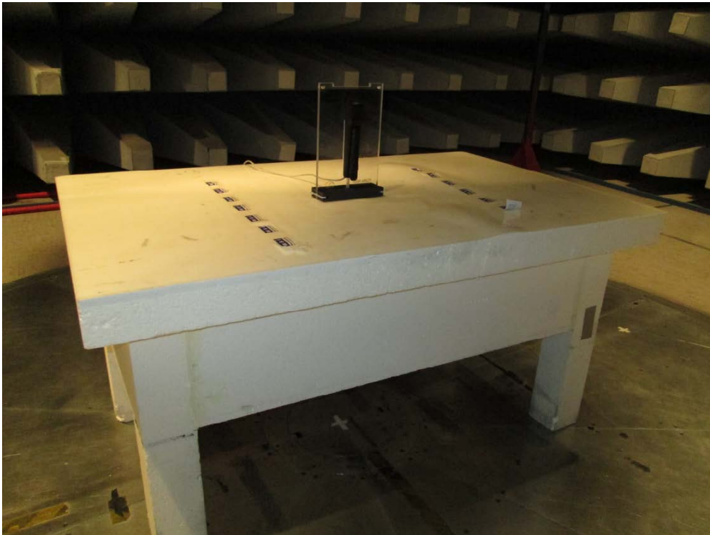
Photo 4.3.1 Test setup regarding measurement of radiated emission 30 – 1000 MHz
