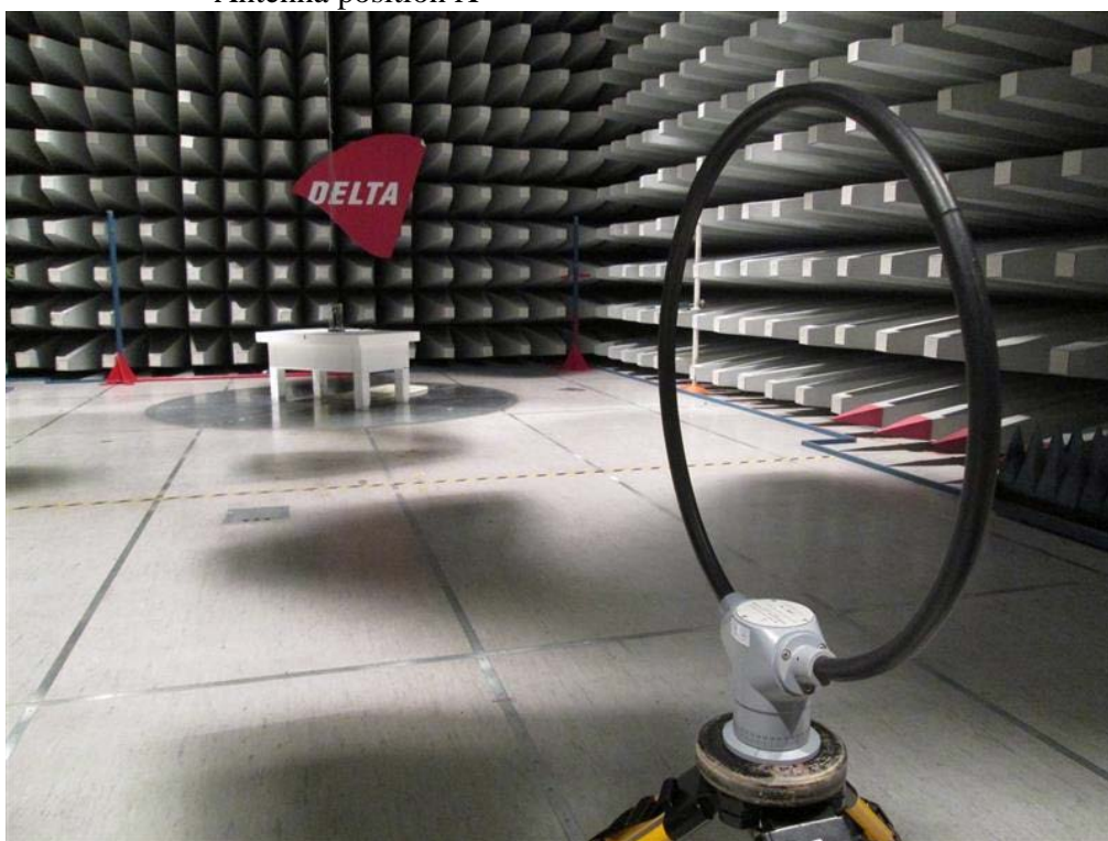
Photo 4.2.2 Test setup regarding measurement of radiated emission 9 kHz – 30 MHz Antenna position Y
