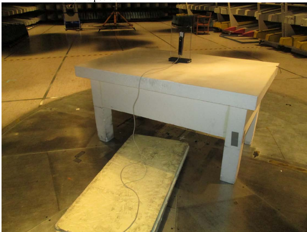
Photo 4.2.4 Test setup regarding measurement of radiated emission 9 kHz – 30 MHz
