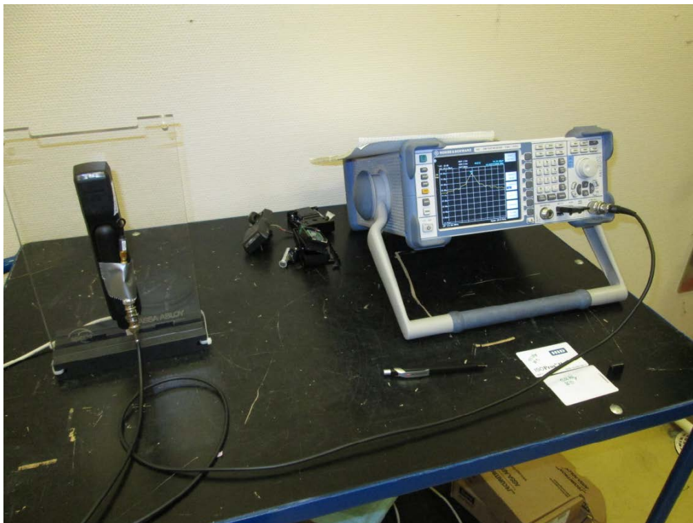
Photo 4.7.1 Test setup regarding measurement of carrier frequency stability.
