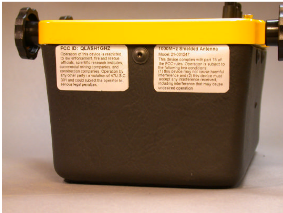
Figure 2. Placement of the FCC labels at the front of the UWB-unit. Visible at all times.
