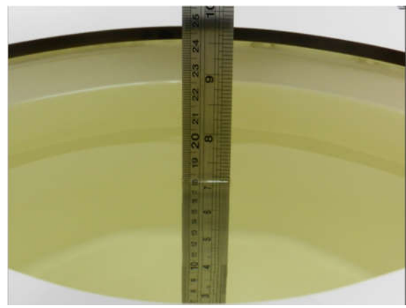
Fig 11.2 Photo of Liquid Height for Body SAR
