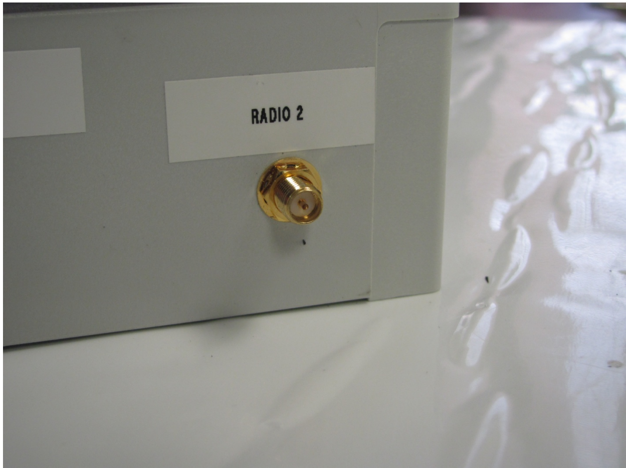
Figure 8. Antenna Port with Antenna Removed (Radio 2)
