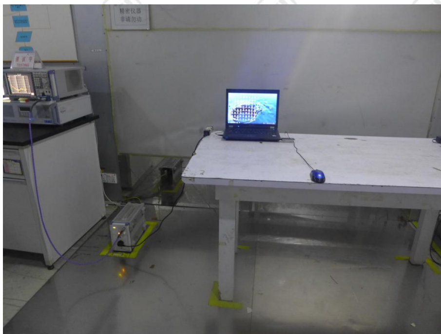
Conducted Emissions Test Setup
