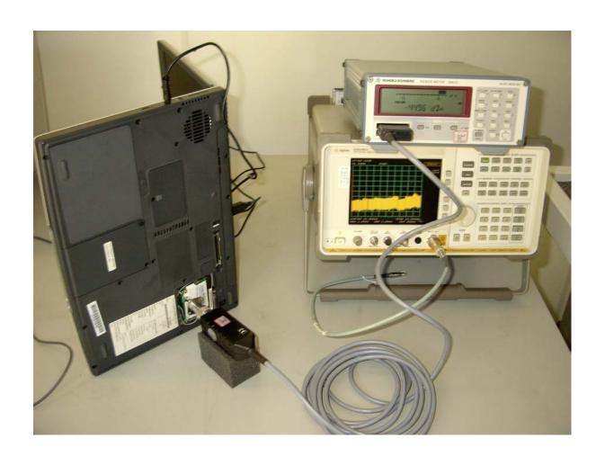
Maximum Peak Output Power Measurement Setup
