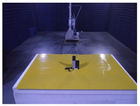
Photo of Radiated Emission Measurement (Above 1G) Powered by adapter
