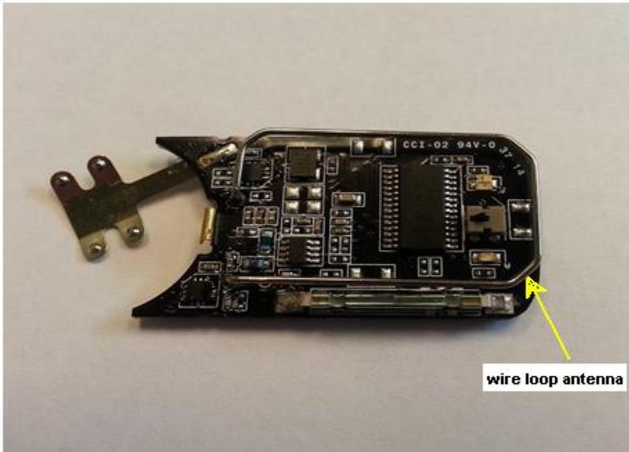
PCB top side and location of "wire loop antenna"
