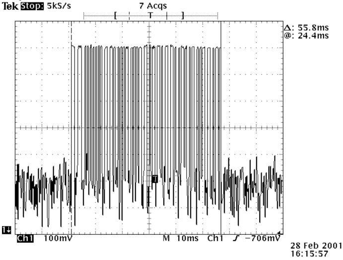
The next two plots show the width of the narrow and wide pulses. The narrow pulses are 0.48ms, and the wide
