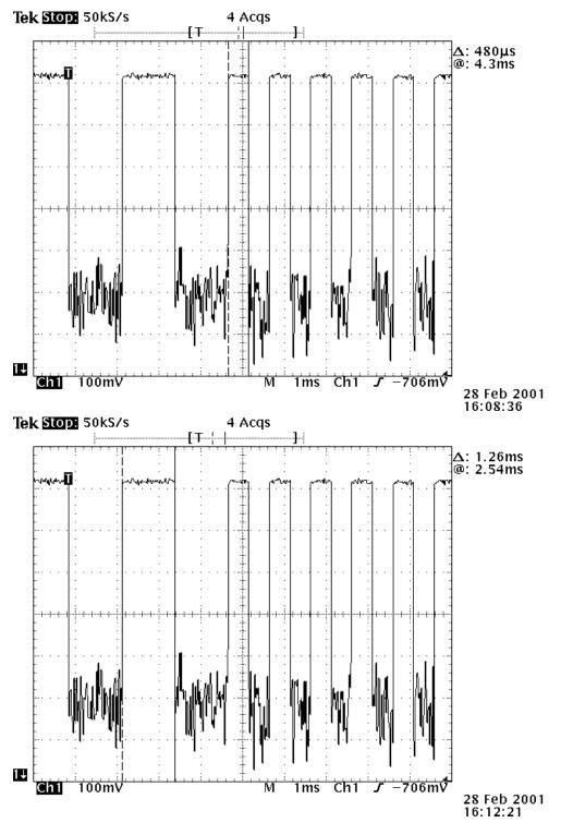
Given 24 narrow peaks of length 0.48ms, and 16 wide peaks of 1.26ms, and a transmission length of 157ms, we
