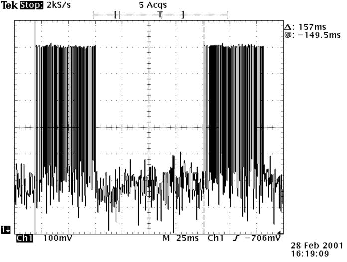
The plot below shows the pulse train. The pulse train duration is 55.8ms. There are 24 narrow peaks and 16 wide peaks.
