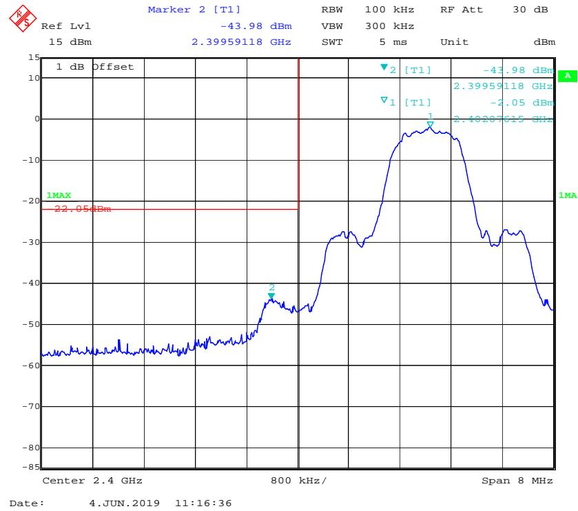
**Band Edge, Right Side**
