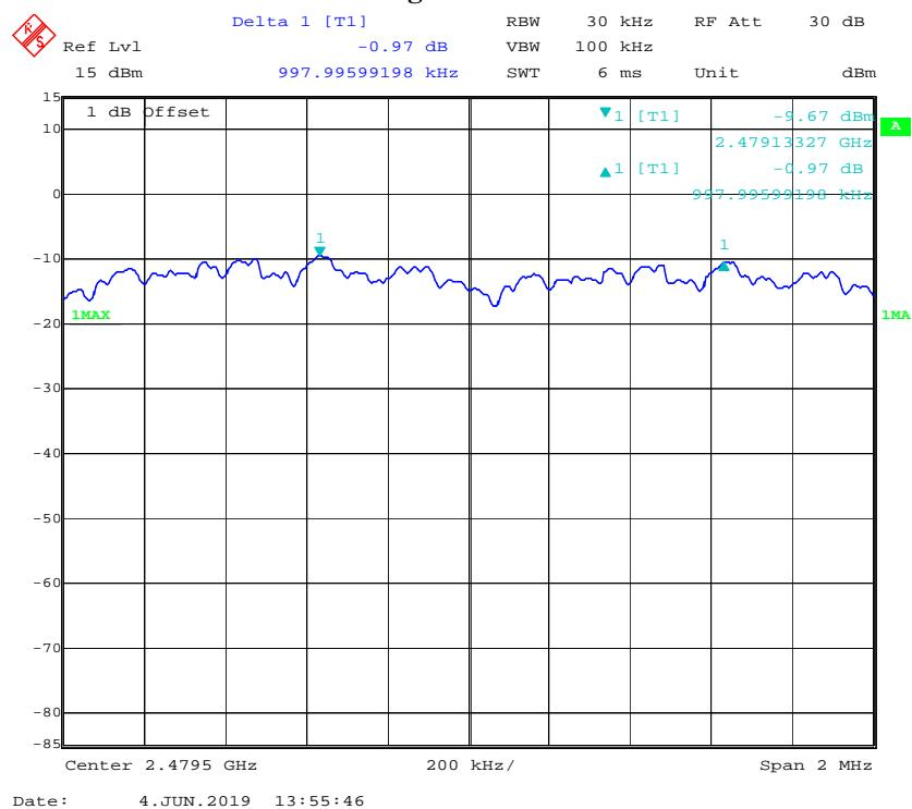
**FCC §15.247(a) (1)–BANDWIDTH TESTING****Applicable Standard**
