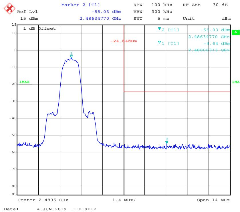
*EDR Mode (8-DPSK):***Band Edge, Left Side**
