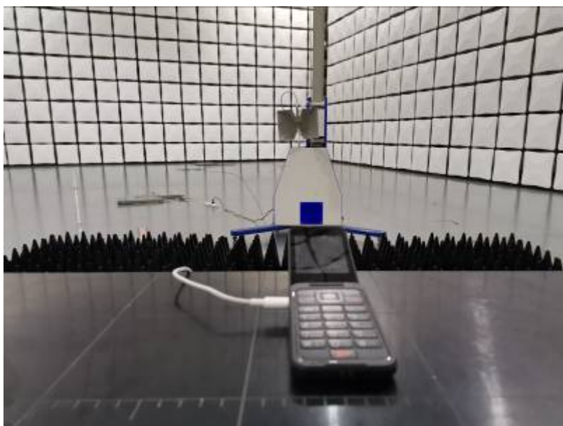
Radiated Emissions Test Setup (above1GHz)
