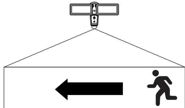
Sensor detects motion that moves across the detection zone
