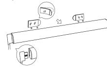
3.Take another "B" segment, connect it with the previous "B" segment that has been installed on the wall, and press it onto the wall for 5 seconds. Then connect "A" segment with the same method.
