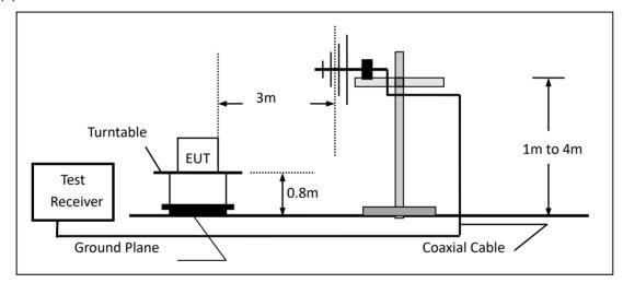
(c) For radiated emissions above 1000MHz
