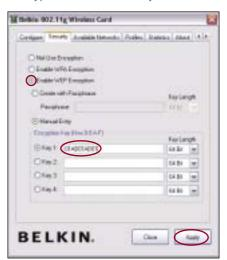
**Important:** A WEP key is a mixture of numbers and letters from A-F and 0-9. For 128-bit WEP, you need to enter 26 keys. For 64-bit WEP, you need to enter 10 keys. This network key needs to match the key you assign to your wireless router (or access point).
