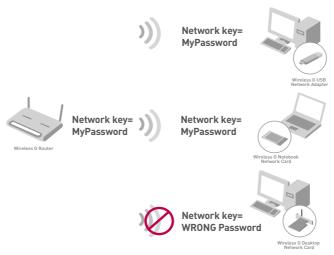
The bottom Card cannot access the network because it uses a different network key than the one configured on the wireless router.
