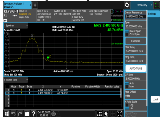
Band Edge_BLE 2M_HighCH39-2480MHz
