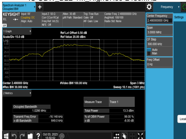
IC OBW_BLE 1M_HighCH39-2480MHz
