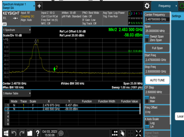
Band Edge_BLE 1M_HighCH39-2480MHz
