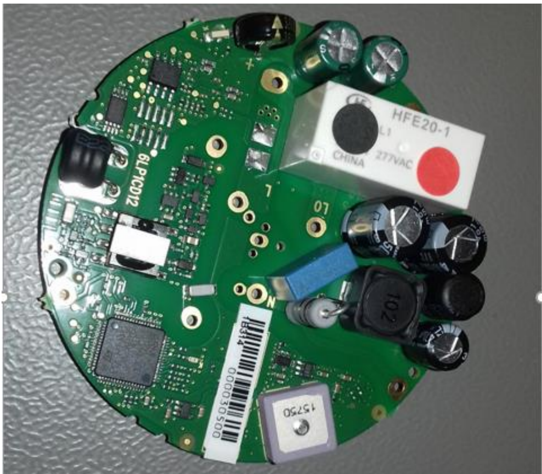
Figure 3 Main PCB top antenna isolator assembly removed
