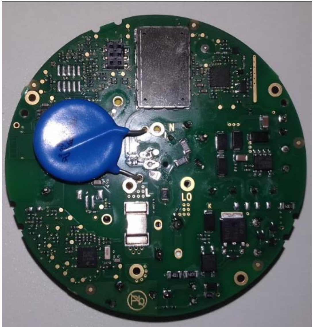
Figure 1 Main PCB bottom with RF screen and varistor fitted
