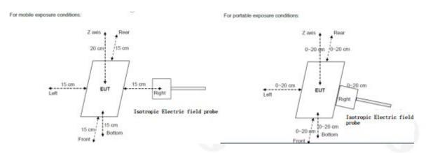
Note: Measurements should be made from all sides and the top of the primary/client pair, with the 20 cm-0cm measured from the center of the top, and 20cm-0cm measured from the center of the rest
