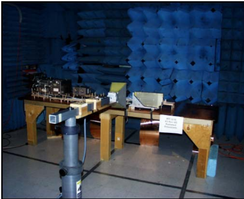
Figure 76. Radiated Emissions Test Setup-MPB
