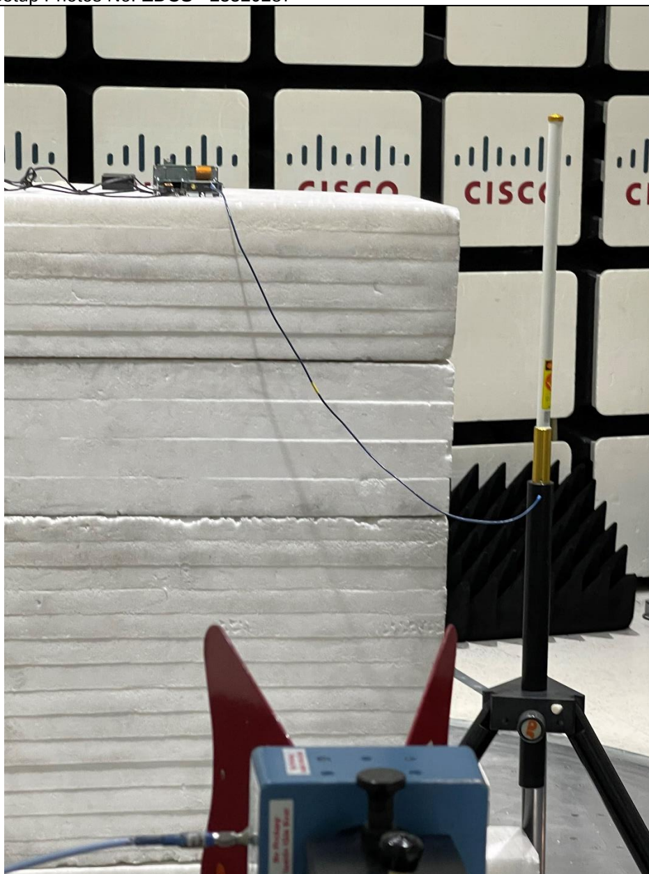
Title: Radiated Spurious Emissions Test Configuration above 1GHz (5.6dBi antenna gain)
