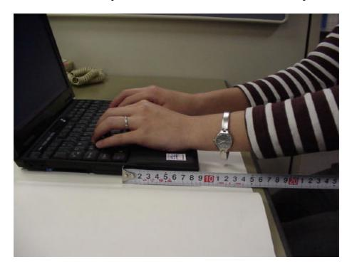
The minimum antenna separation to satisfy the MPE limits (1mW/cm²), and the maximum power density in 20cm distance of each card are :
