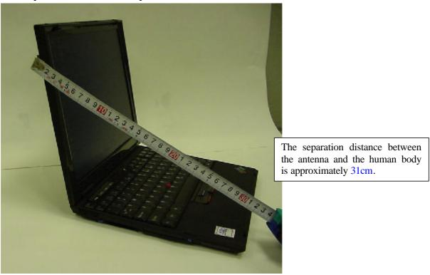
The peak conducted output power of the applying equipment is 15.3dBm and the maximum antenna gain is -0.38dBi as shown below.
