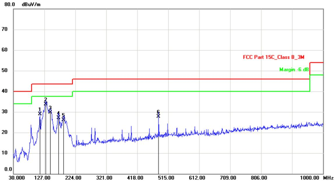
Site Polarization: *Horizontal* Temperature: 26
