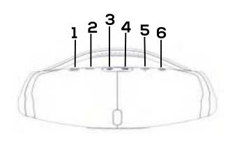
1: Press to switch between modes (Bluetooth / Radio). 2: Short press to previous song / Long press to volume
