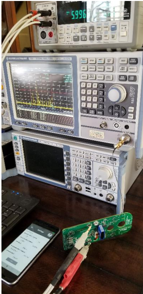
Figure 5: Conducted RF Test Setup Photograph(s).
