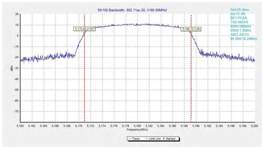
Fig.63 99% Occupied bandwidth (802.11ac-HT20, 5180MHz)
