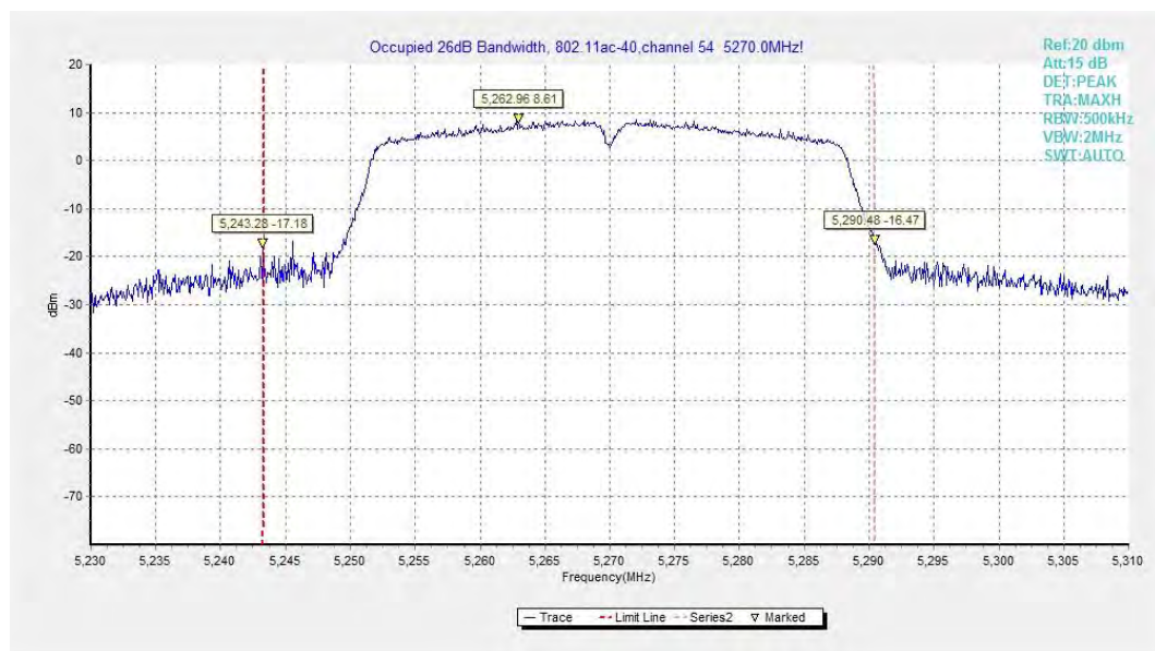
Fig.23 Occupied 26dB Bandwidth (802.11ac-HT40, 5270MHz)
