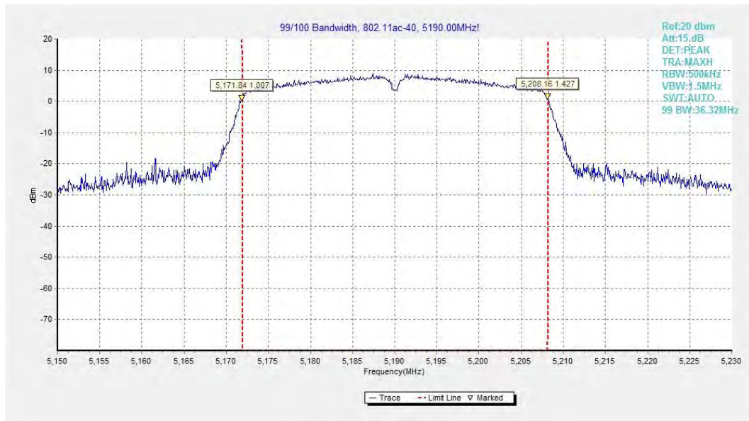
Fig.66 99% Occupied bandwidth (802.11ac-HT40, 5190MHz)
