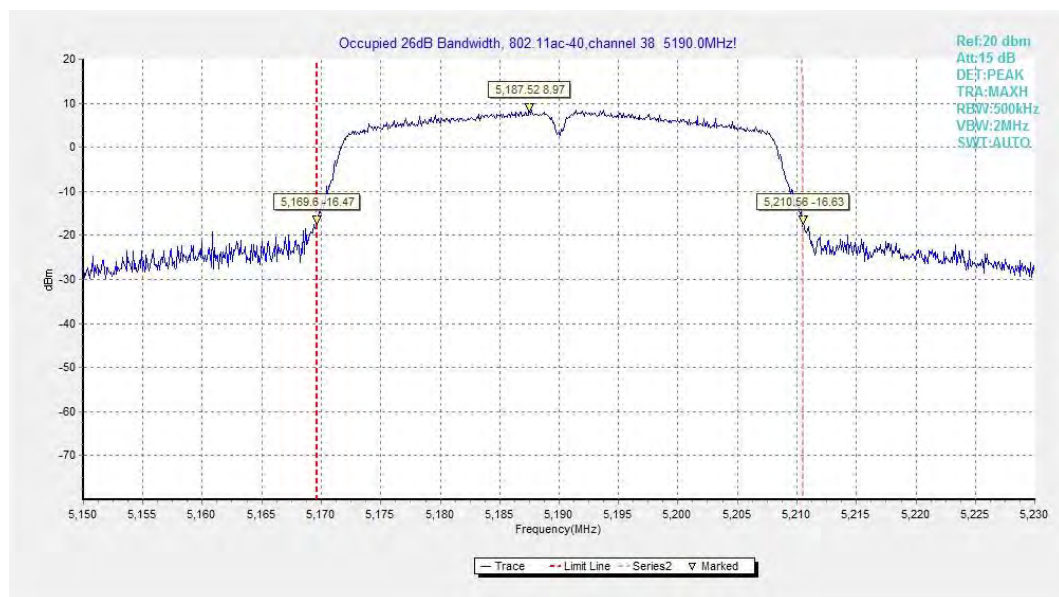
Fig.21 Occupied 26dB Bandwidth (802.11ac-HT40, 5190MHz)
