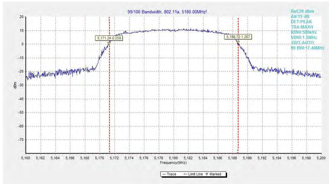
Fig.60 99% Occupied bandwidth (802.11a, 5180MHz)
