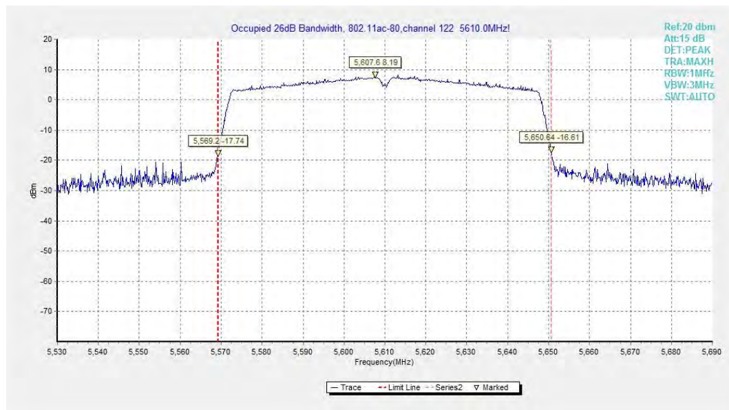
Fig.32 Occupied 26dB Bandwidth (802. 11ac-HT80, 5610MHz)
