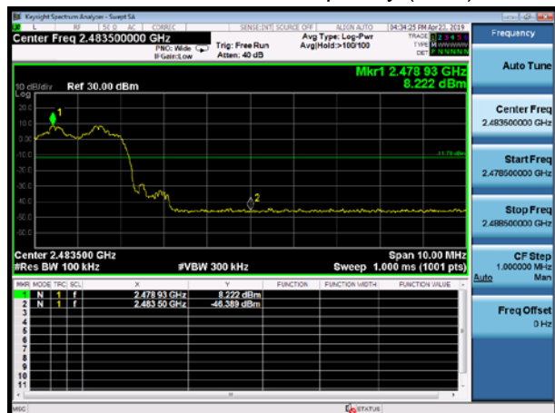
BT 3DH5 CH78, Carrier frequency (MHz): 2480
