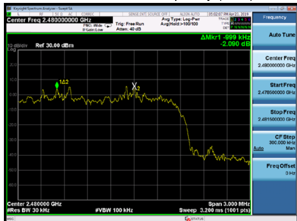
BT 2DH5 CH78, Carrier frequency (MHz): 2480
