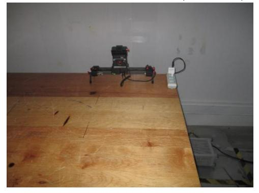
8.2 Field Strength of the Fundamental Signal (15.249(a)) Test Setup
