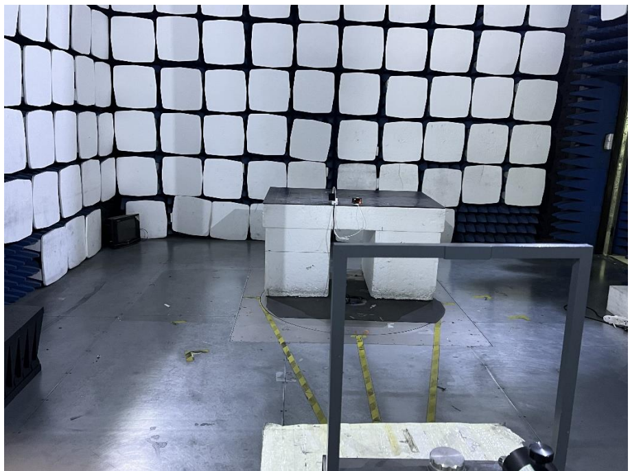
Radiation Emission Test Setup (Below 30MHz)
