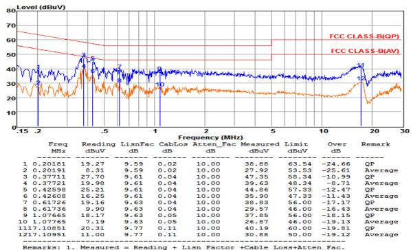
Remarks: 1. Measured = Reading + Lisn Factor +Cable Loss+Atten\_Fac.
