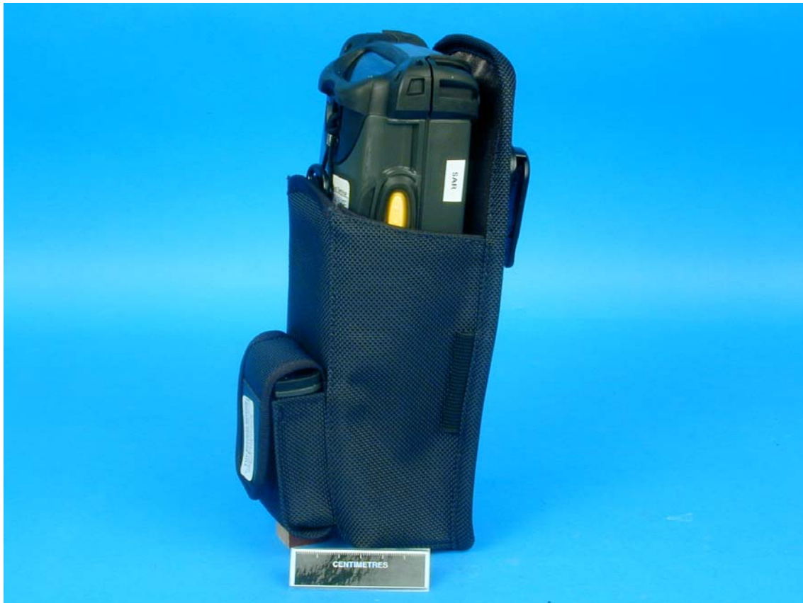
Figure 43. Device placed in correct position with the MC9062 Mobile Computer Holster with LCD facing rear of Holster.
