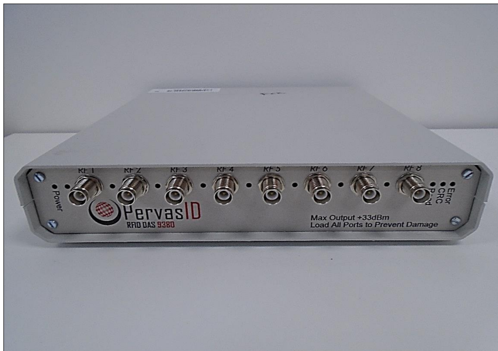
Figure 1 – EUT Front View - SRM 9380 (8-port Master)
