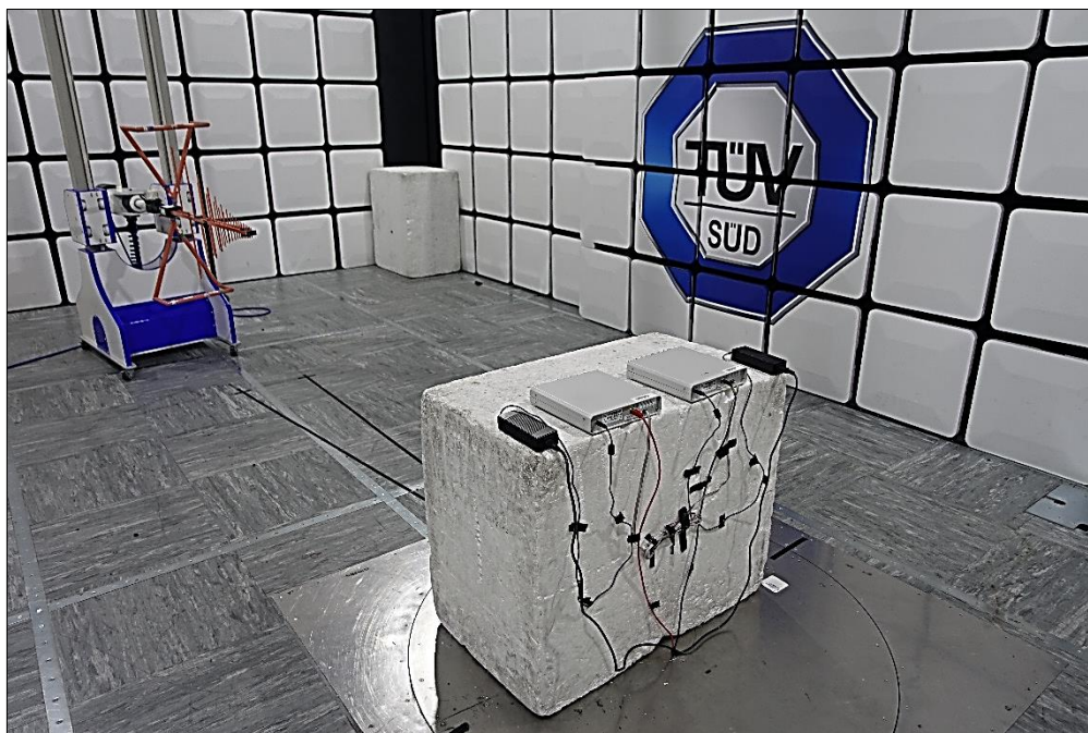
Figure 9 - Test Setup - 30 MHz to 1 GHz
