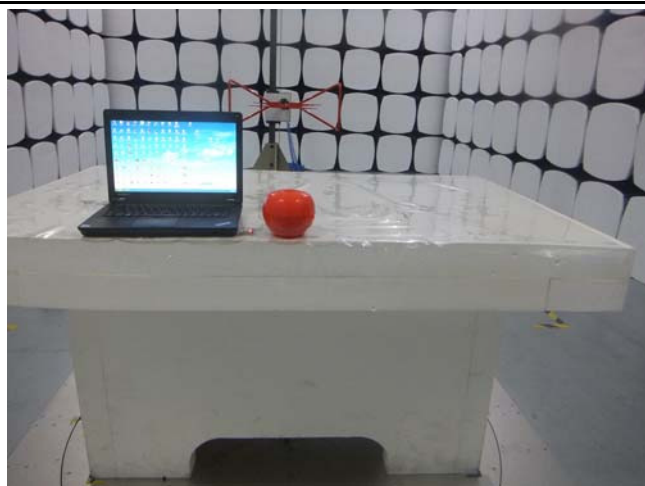
Radiated Spurious Emissions Test Setup Below 1GHz
