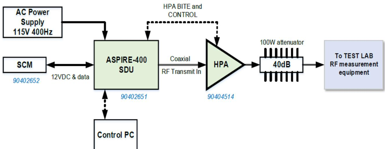
**Note:** To test the SDU RF power a directional coupler was used between the SDU and HPA and the 20 dB coupling port was used to measure the power and mask requirements. All other measurements were taken from the HPA output.
