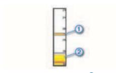
The a-scope above shows fish returns  $\bigcirc$  and a soft bottom return  $\bigcirc$ .
