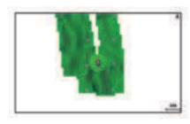
A green circle indicates good depth and GPS position, and a speed under 16 km/h (10 mph). A yellow circle indicates good depth and GPS position, and a speed between 16 and 32 km/h (10 and 20 mph). A red circle indicates poor depth or GPS position, and a speed above 32 km/h (20 mph).
