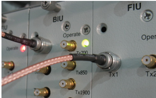
Figure 24 BTS QMA Coaxial Cable Connection
