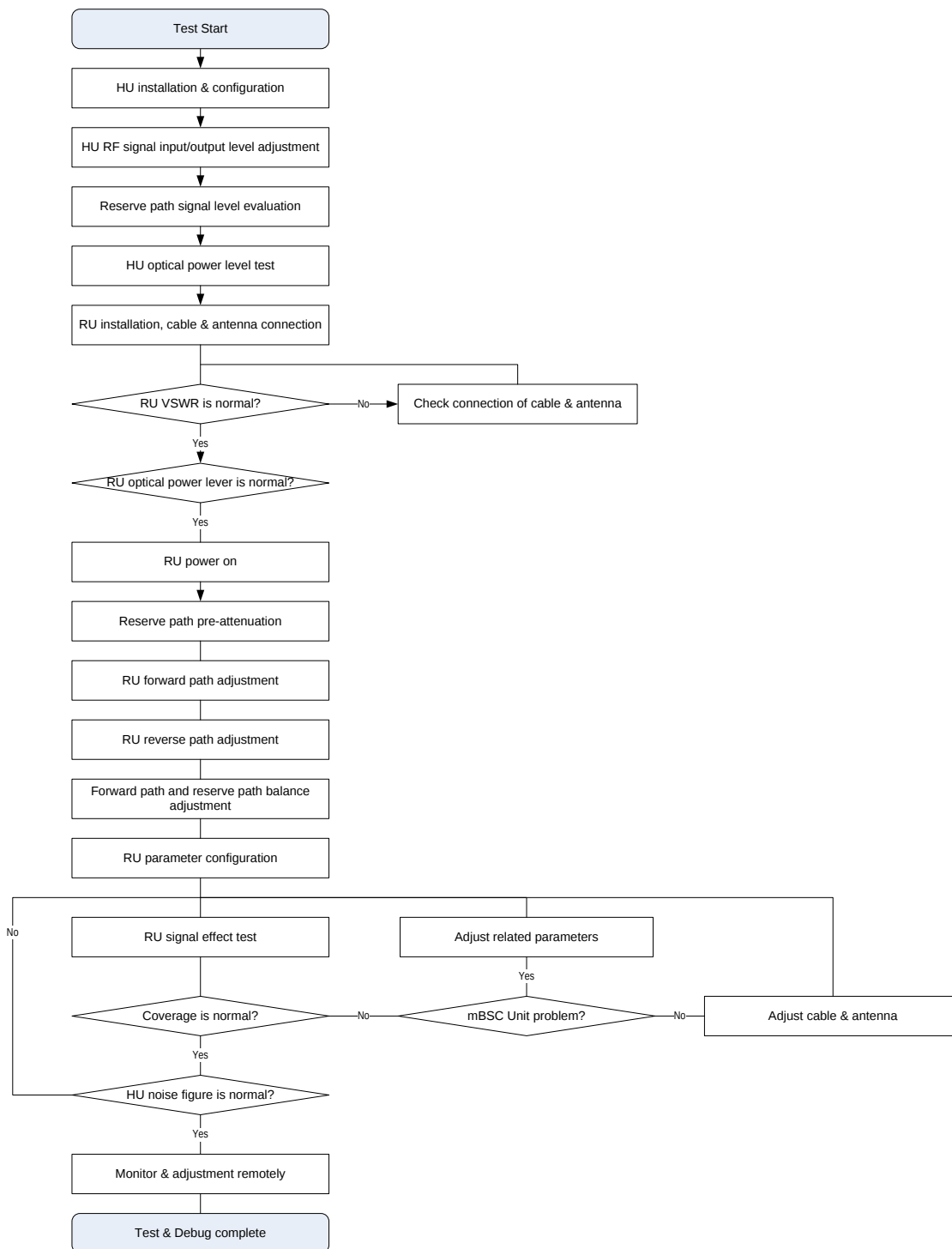
Figure 36 Flow Chart of System Debugging
