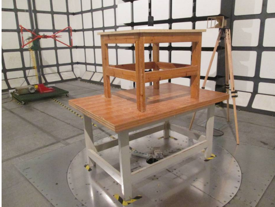
Radiated Emissions Test View (Below 1 GHz)
