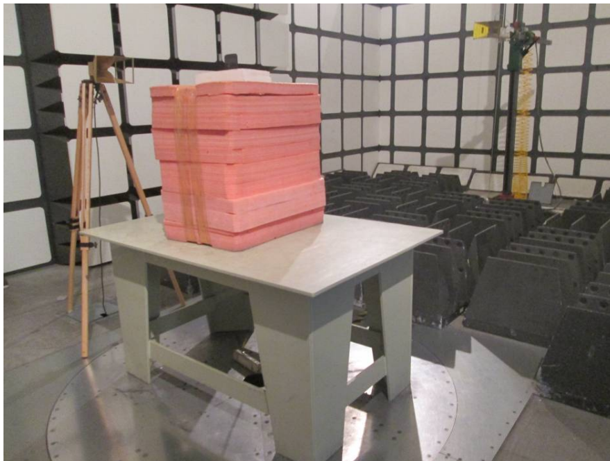
Radiated Emissions Test View (Above 1 GHz)
