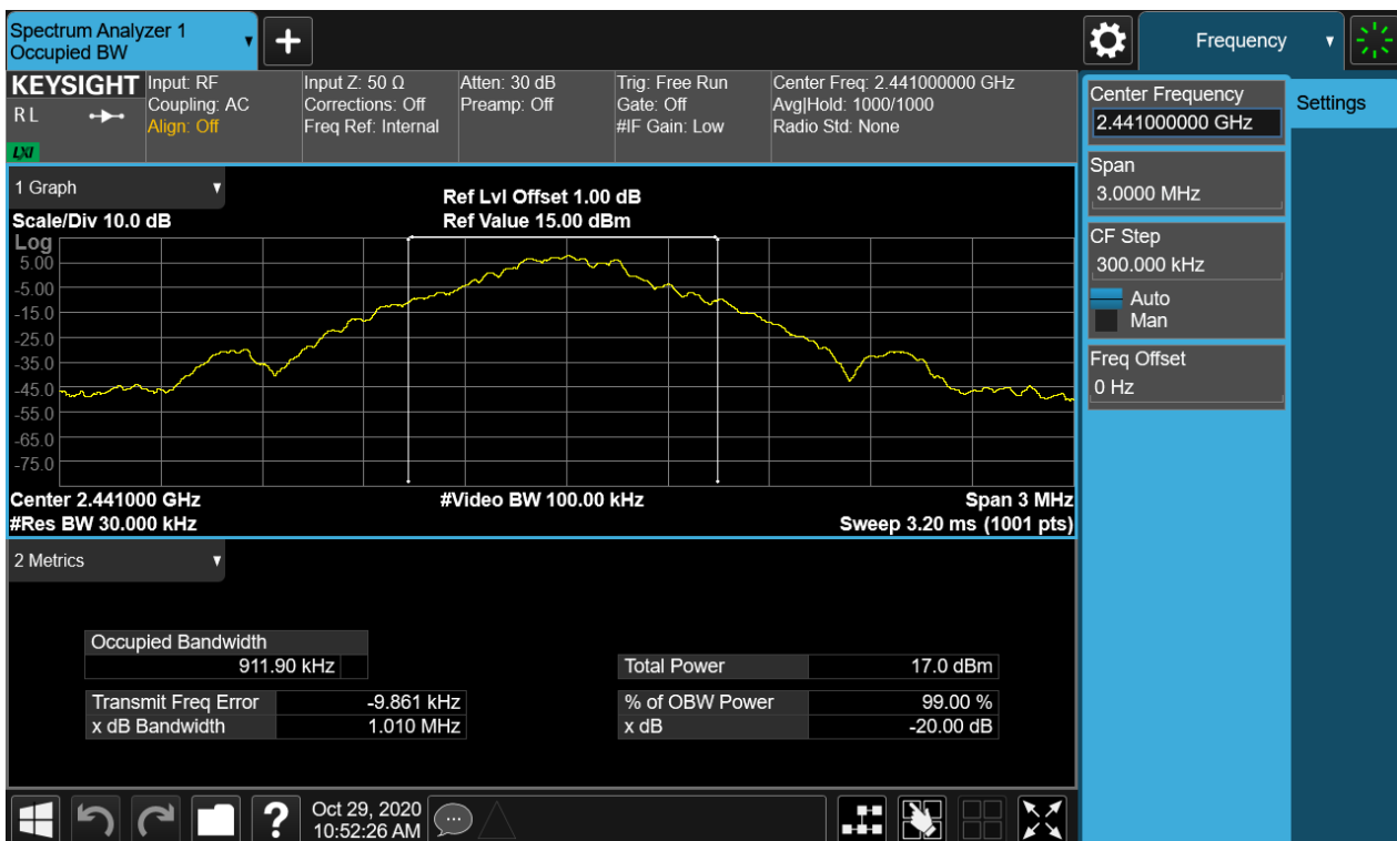
Figure 11: 20dB Bandwidth and 99% Bandwidth, 2441MHz, GFSK
