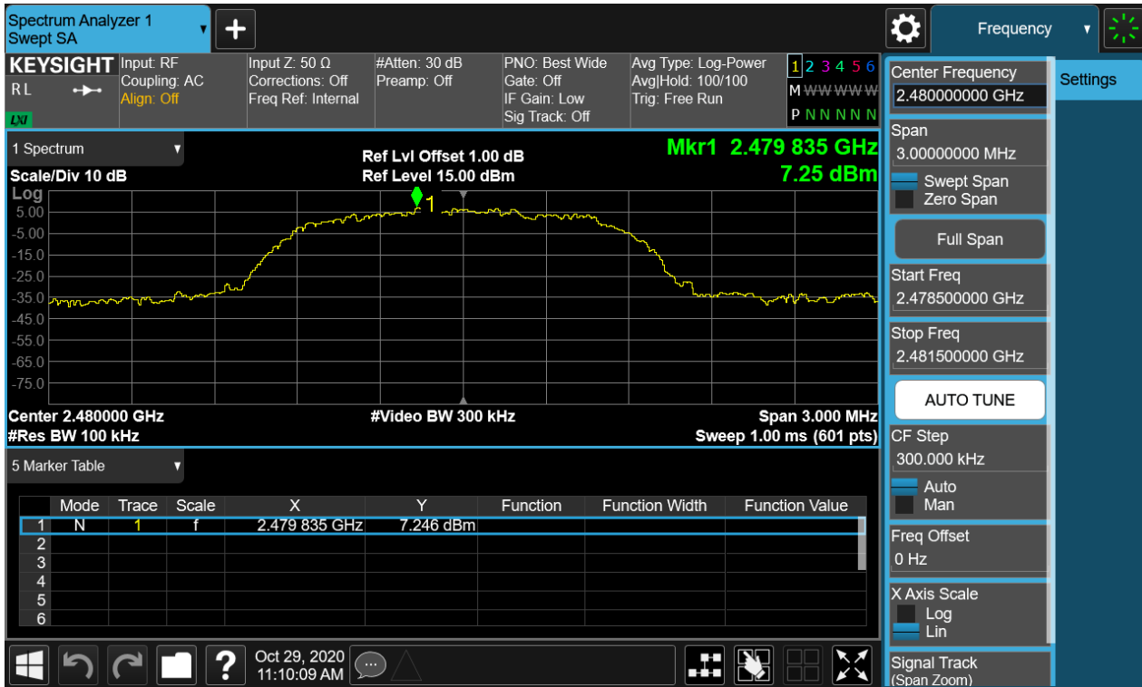
Figure 21: Conducted Spurious Emission & Authorized-band band-edge, 2480MHz, 8-DPSK Carrier Level
