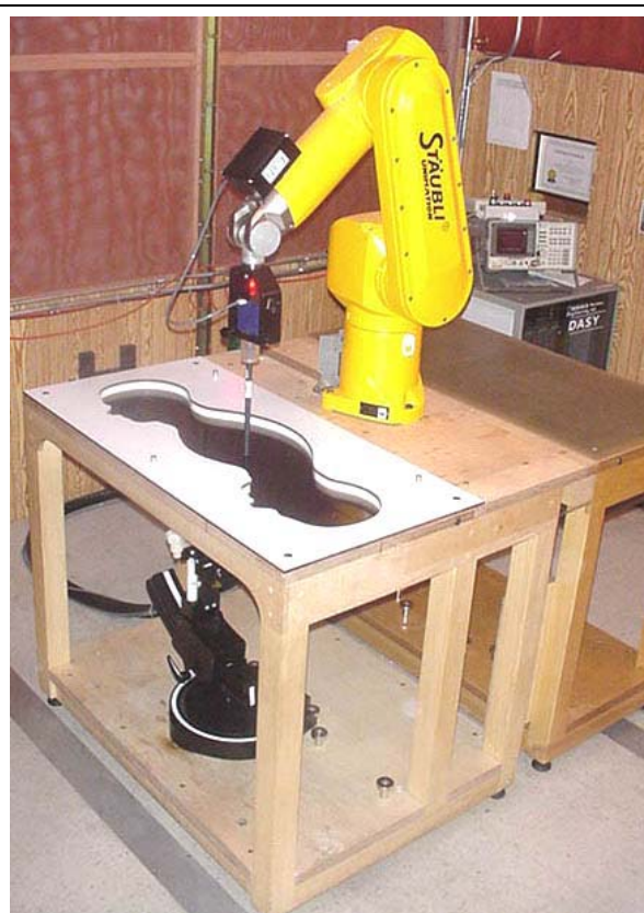
DASY4 Measurement System with SAM Phantom and device holder
