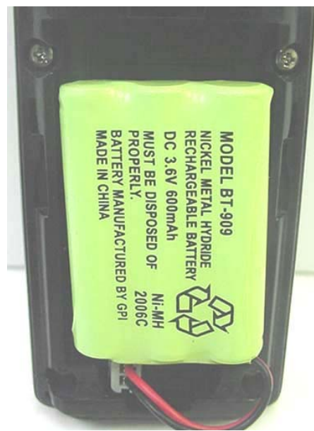
Ni-MH Battery 3.6V, 600mAh
