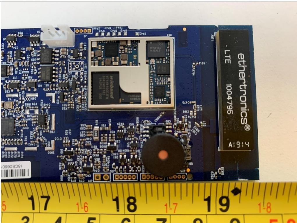
EUT Cover Off View-Top without shielding
