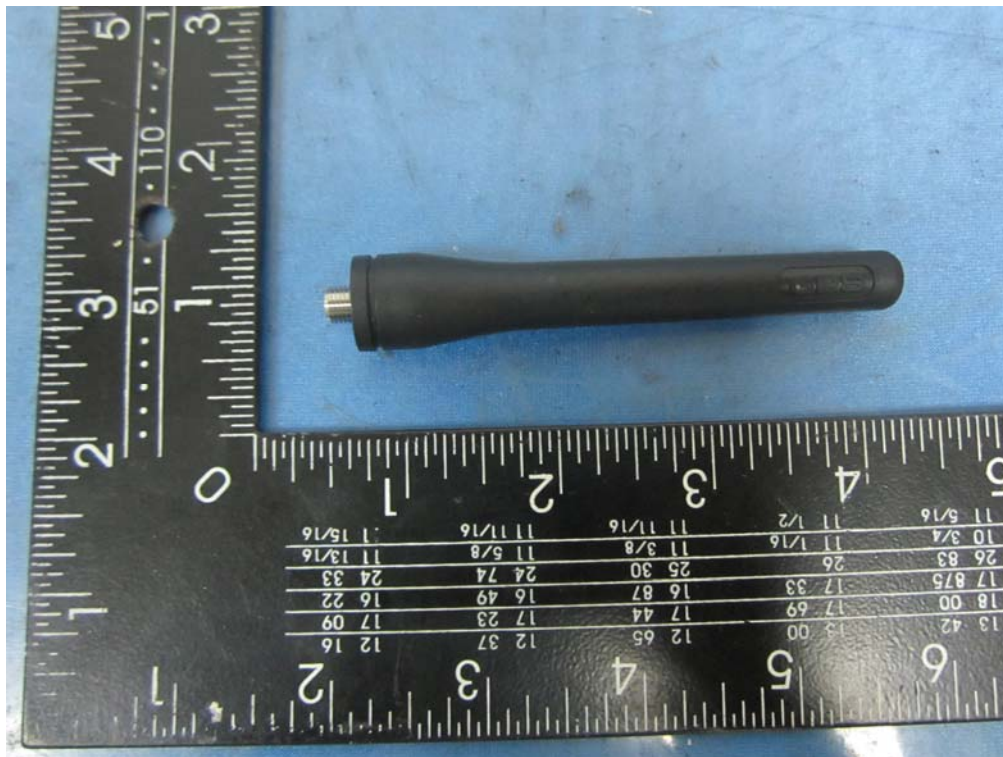
A1- Antenna,400-470 MHz,Stub,DMR: AN0435H05
