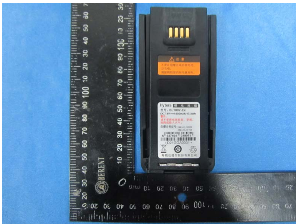
B1- Battery, Intrinsically Safe Li-ion Battery(1800mAh): BL1807-Ex
