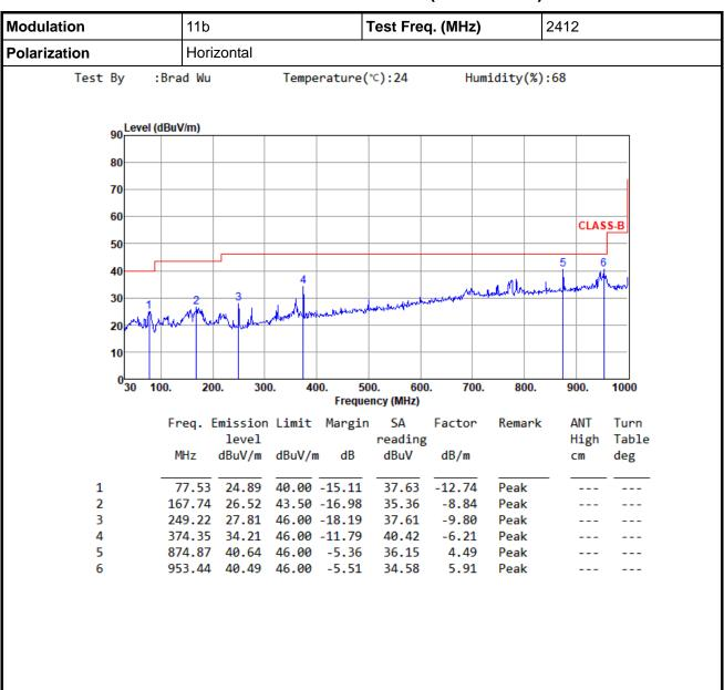
Note 1: Emission Level (dBuV/m) = SA Reading (dBuV) + Factor\* (dB/m)
