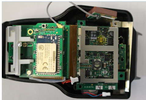
Pic 6 – BI LOC8 GSM nested board installed
