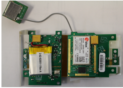
Pic 4 – BI LOC8 GSM Nested Board – 150mAh battery (Left), Cell, GSM module (Right)
