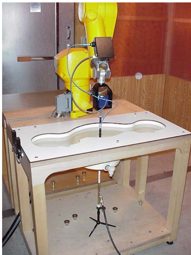
DASY4 SAR Measurement System with SAM phantom & validation dipole
