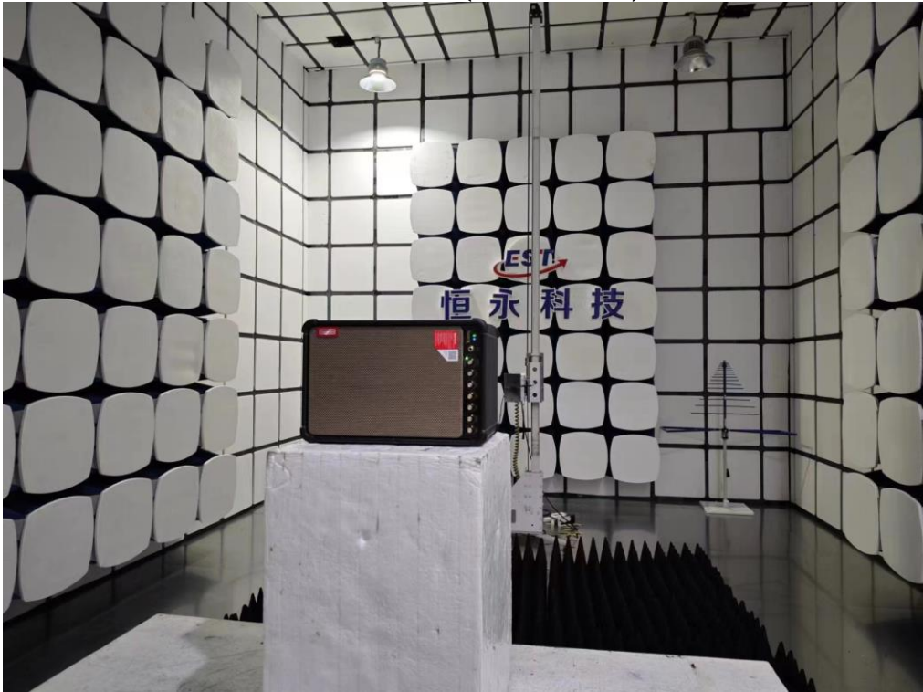
Radiated Test (Above 1GHz)
