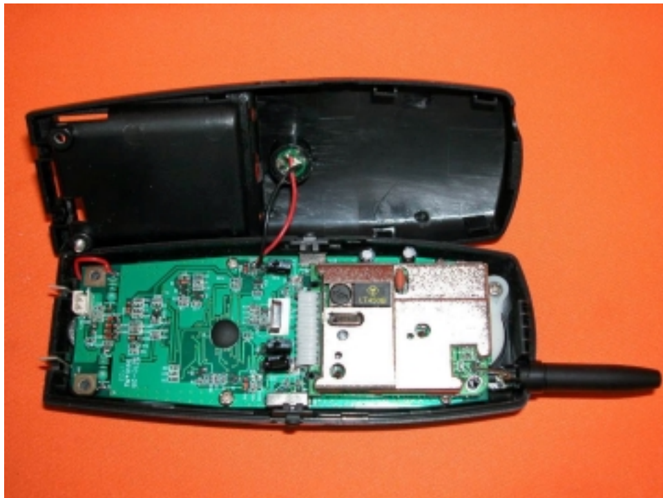
Handset Main PCB comp side (View 1)
