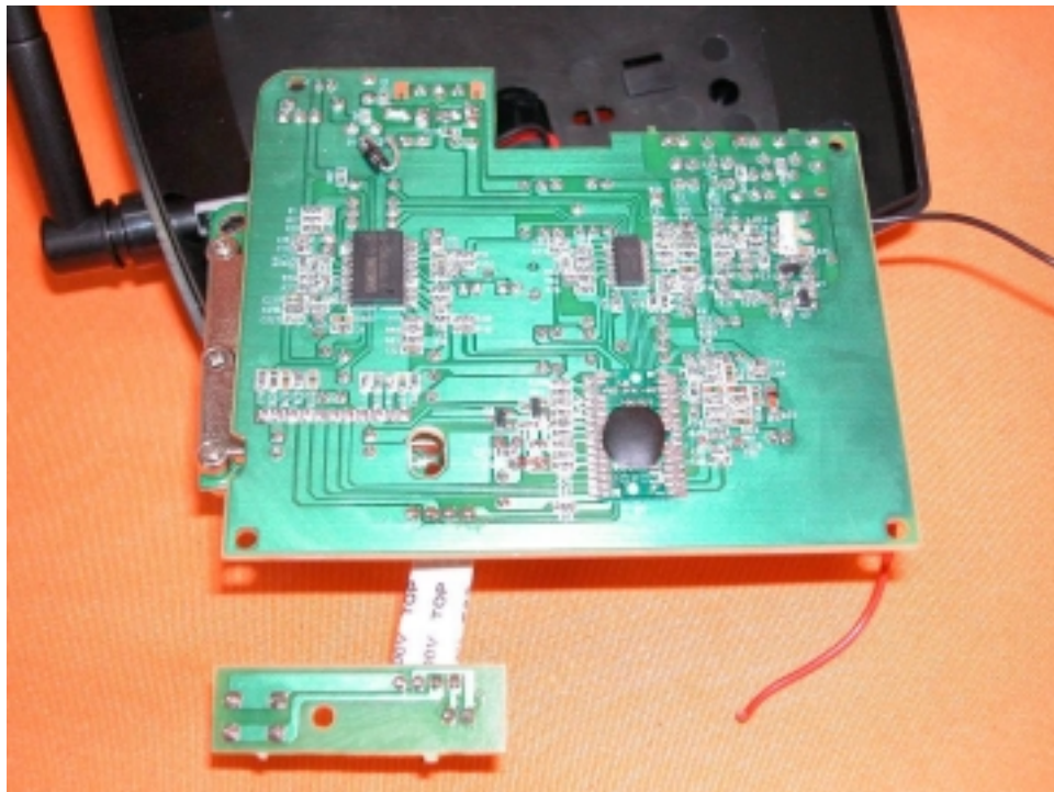
Base Main PCB solder side
