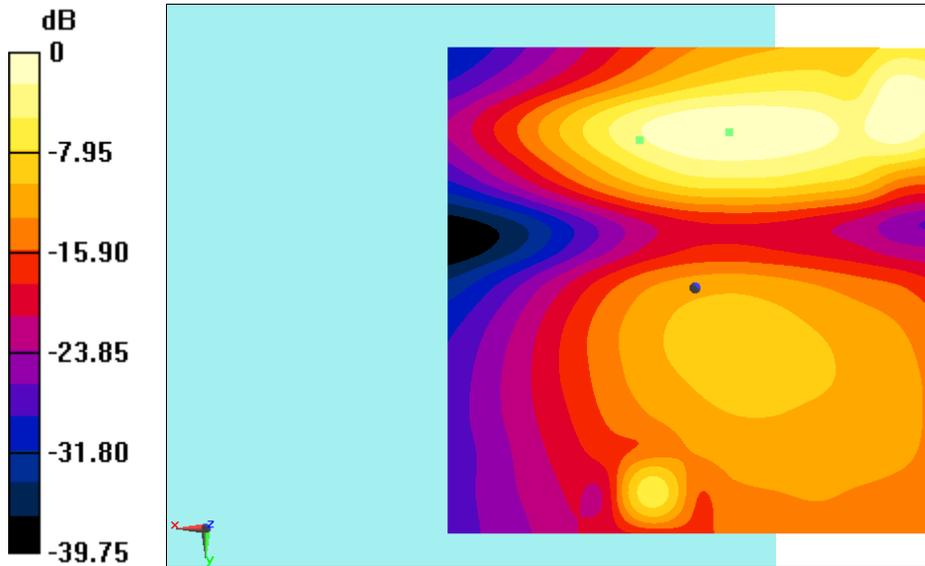
$0 \text{ dB} = 0.3737 \text{ A/m} = -8.55 \text{ dBA/m}$ **Fig B.1 T-Coil LTEB41**
