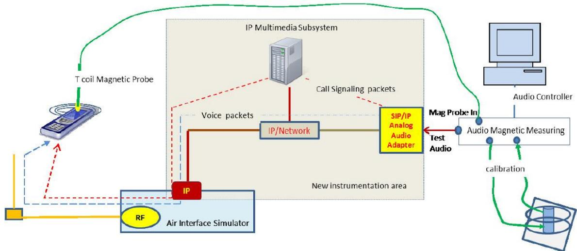
**Figure 10.1 Test Setup for VoWiFi over IMS T-coil Measurements**
