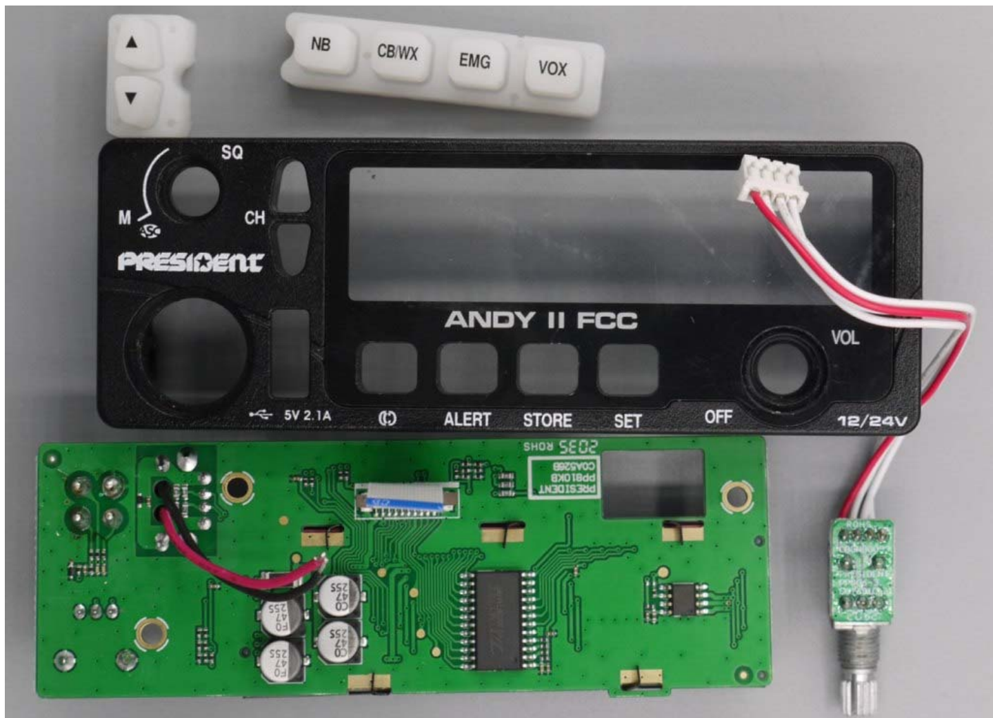
Figure E20.4 – Internal Photo – Front Assembly – Front View
