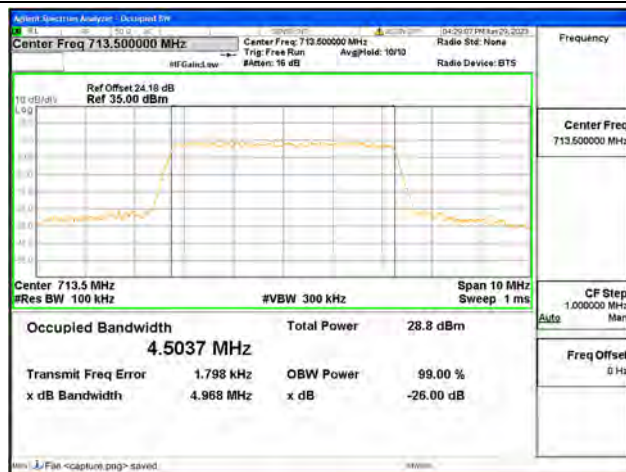
Band12 / 5MHz / 64QAM/ High CH
