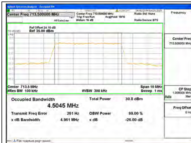
Band17 / 5MHz / QPSK/ High CH
