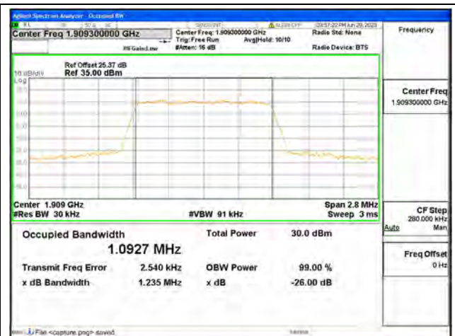
Band2 / 1.4MHz / 16QAM/ High CH
