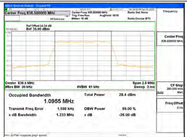
Band5 / 1.4MHz / 64QAM/ Mid CH
