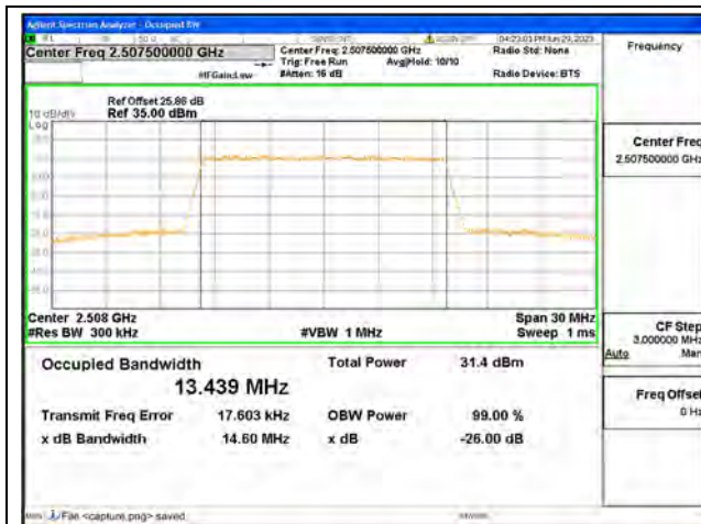
Band7 / 15MHz / QPSK/ Low CH
