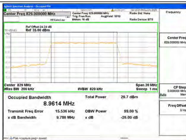
Band5 / 10MHz / 16QAM/ Low CH
