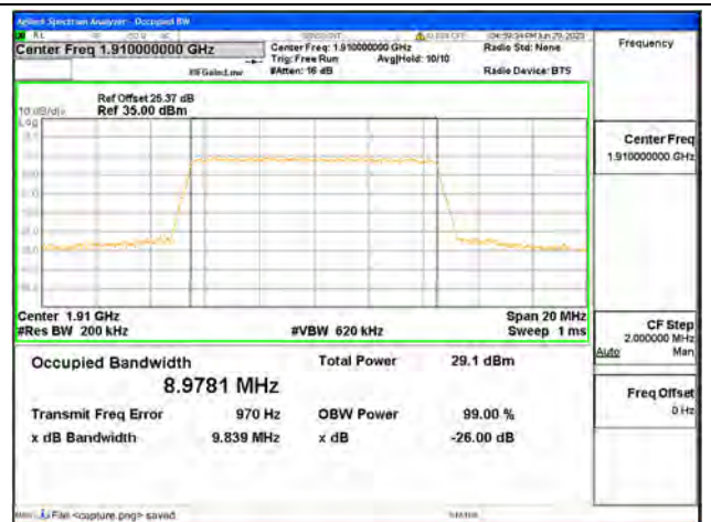
Band25 / 10MHz / 64QAM/ High CH
