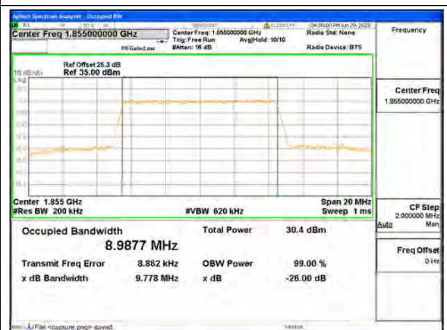
Band2 / 10MHz / 64QAM/ Low CH
