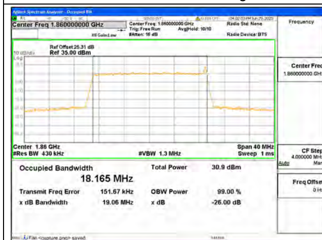
Band2 / 20MHz / 16QAM/ Low CH
