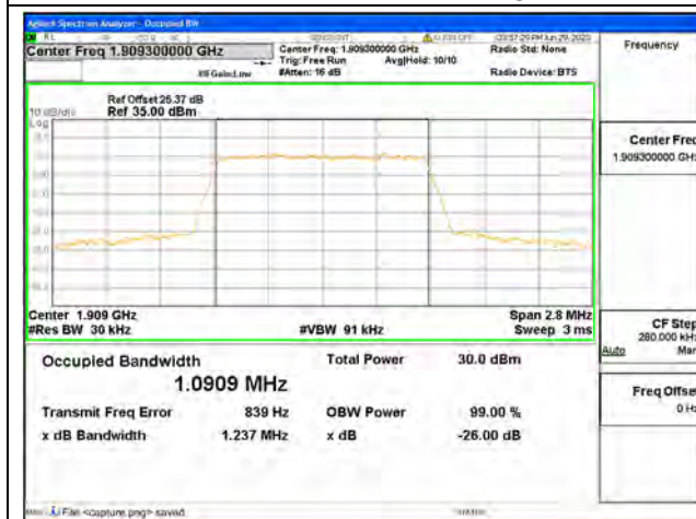
Band2 / 1.4MHz / 64QAM/ High CH
