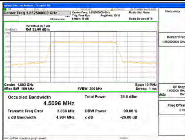
Band25 / 5MHz / 64QAM/ Low CH
