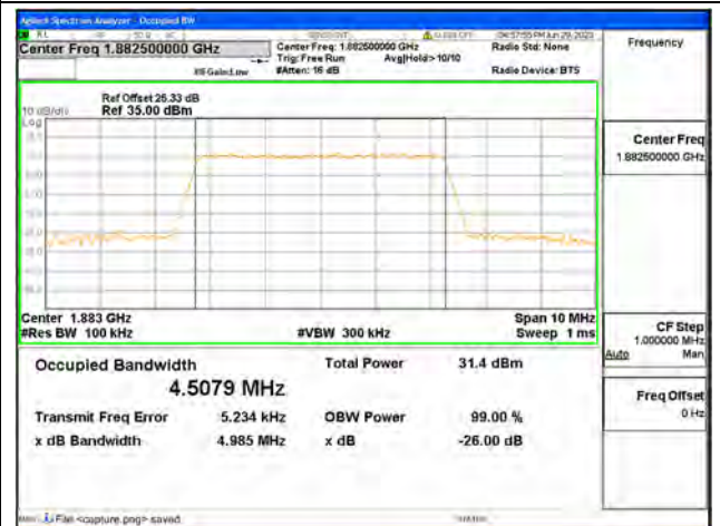
Band25 / 5MHz / QPSK/ Mid CH
