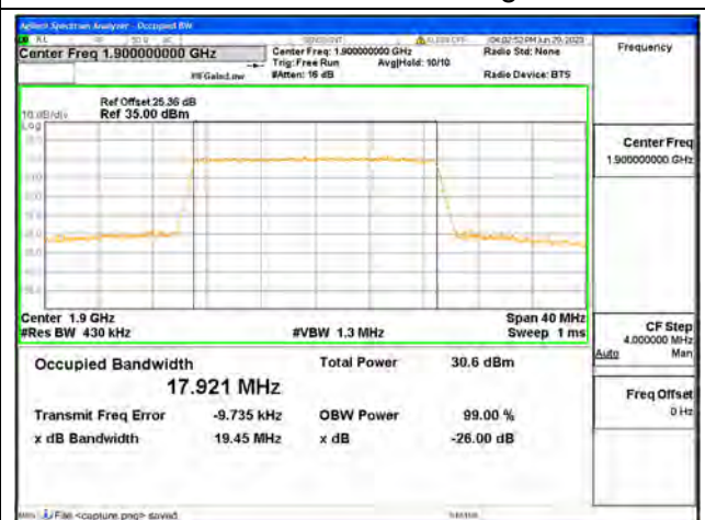
Band2 / 20MHz / 64QAM/ High CH
