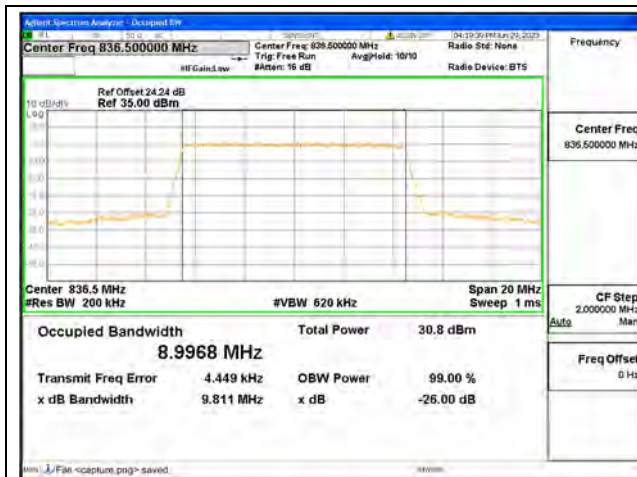
Band5 / 10MHz / QPSK/ Mid CH
