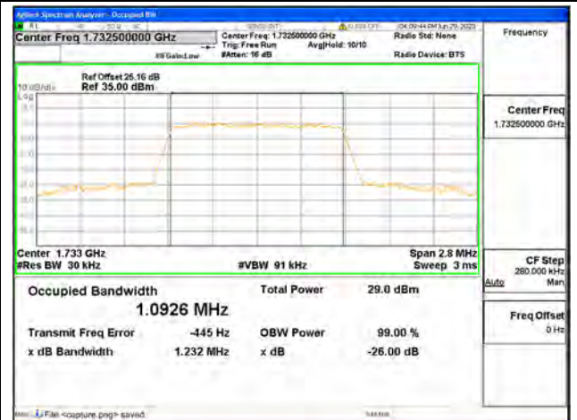
Band4 / 1.4MHz / 64QAM/ Mid CH
