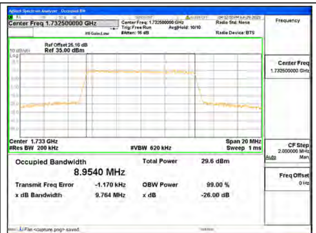
Band4 / 10MHz / 16QAM/ Mid CH
