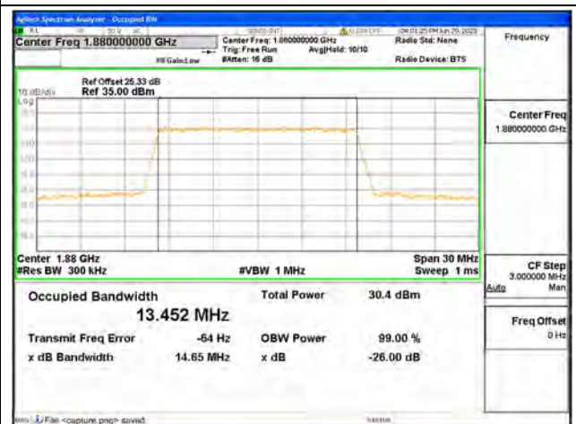
Band2 / 15MHz / 64QAM/ Mid CH
