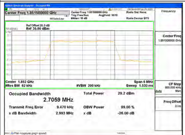
Band25 / 3MHz / 64QAM/ Low CH
