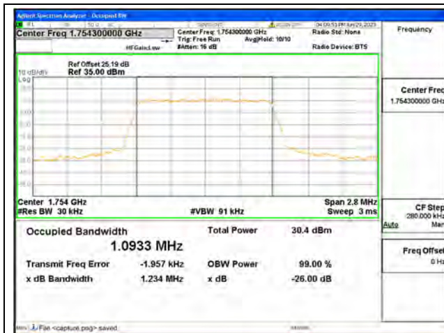
Band4 / 1.4MHz / QPSK/ High CH
