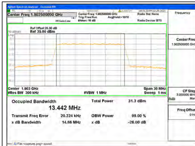
Band2 / 15MHz / QPSK/ High CH
