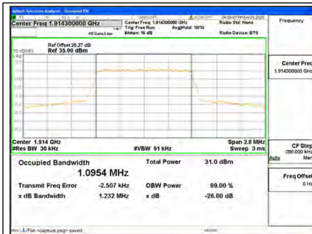
Band25 / 1.4MHz / QPSK/ High CH
