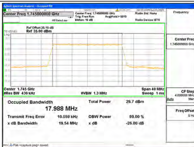
Band4 / 20MHz / 16QAM/ High CH
