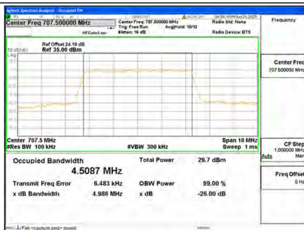
Band12 / 5MHz / 16QAM/ Mid CH
