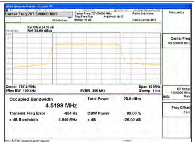
Band12 / 5MHz / 64QAM/ Mid CH
