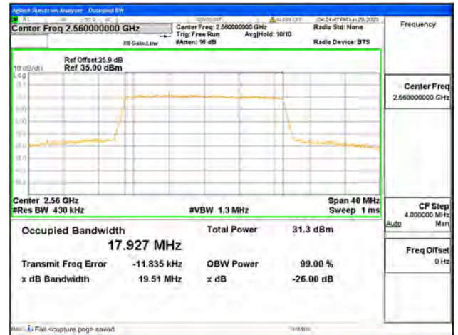
Band7 / 20MHz / QPSK/ High CH
