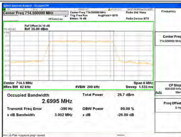
Band12 / 3MHz / 16QAM/ High CH
