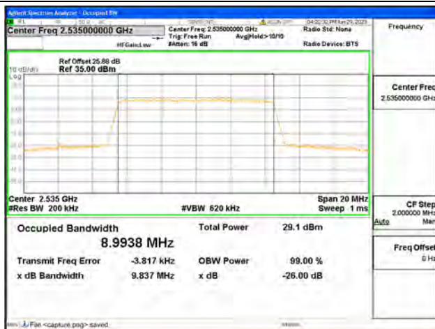
Band7 / 10MHz / 64QAM/ Mid CH
