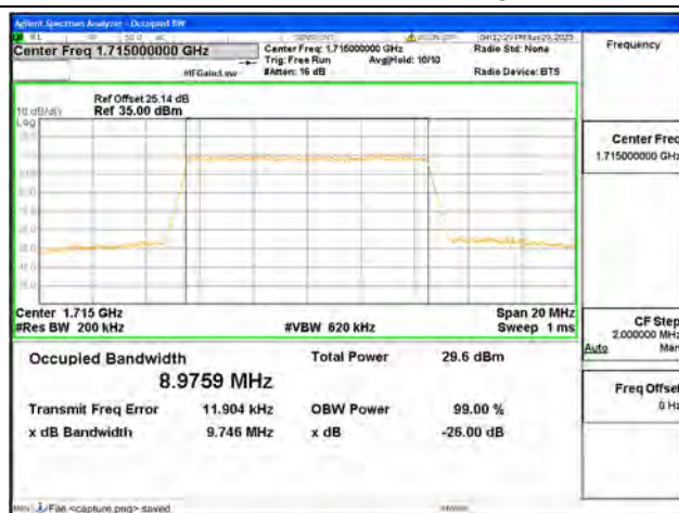
Band4 / 10MHz / 16QAM/ Low CH
