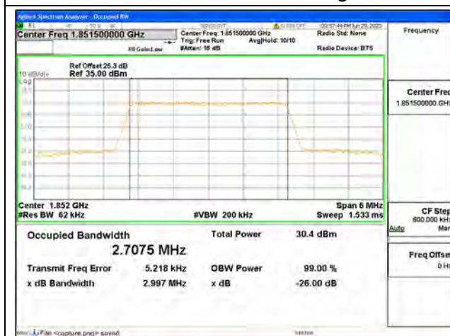
Band2 / 3MHz / 16QAM/ Low CH
