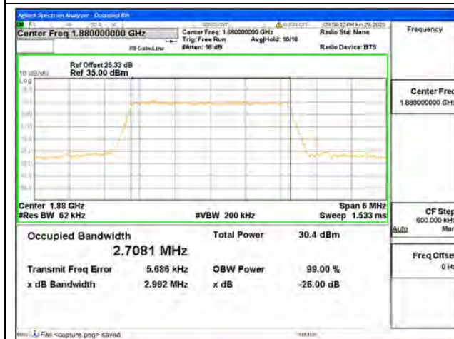
Band2 / 3MHz / 64QAM/ Mid CH
