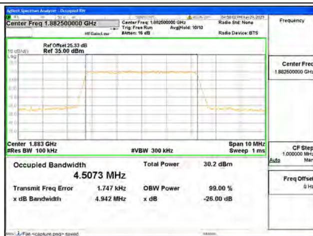
Band25 / 5MHz / 16QAM/ Mid CH
