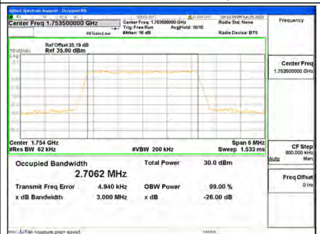
Band4 / 3MHz / 64QAM/ High CH
