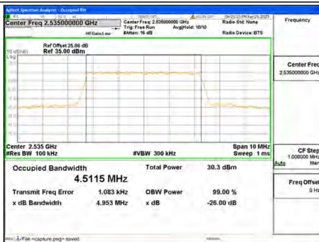
Band7 / 5MHz / 16QAM/ Mid CH
