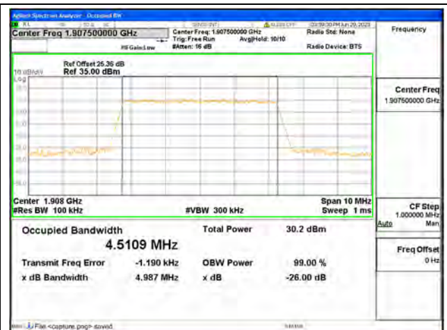
Band2 / 5MHz / 16QAM/ High CH
