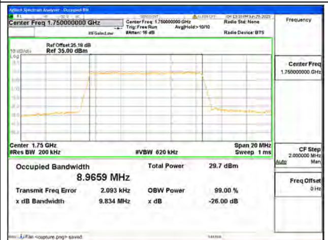
Band4 / 10MHz / 64QAM/ High CH
