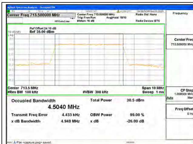
Band12 / 5MHz / QPSK/ High CH
