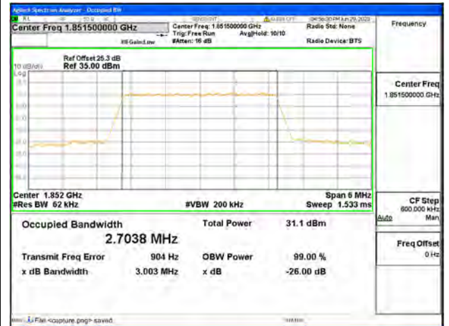
Band25 / 3MHz / QPSK/ Low CH
