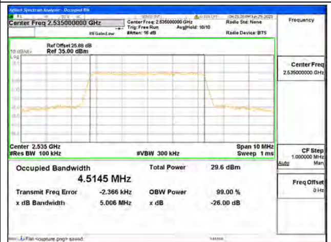
Band7 / 5MHz / 64QAM/ Mid CH
