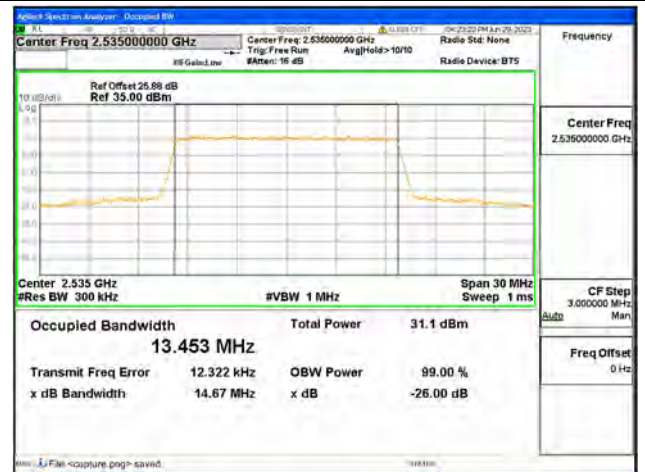
Band7 / 15MHz / QPSK/ Mid CH
