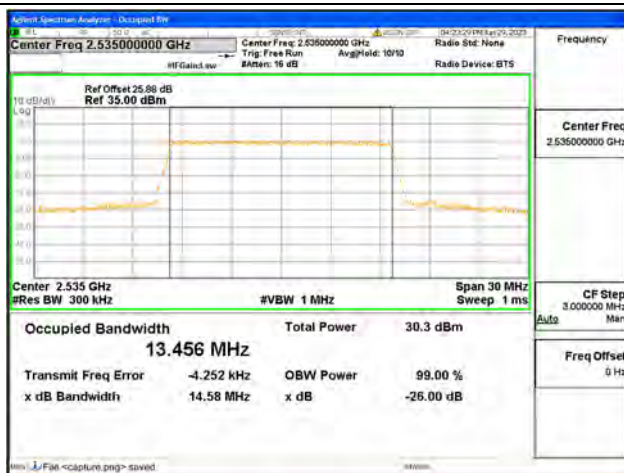
Band7 / 15MHz / 16QAM/ Mid CH
