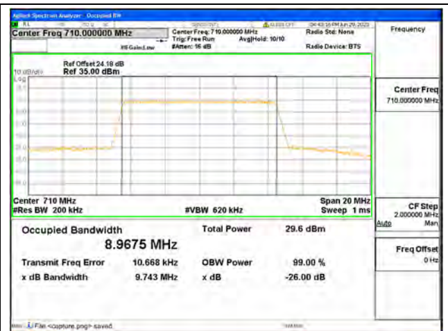
Band17 / 10MHz / 16QAM/ Mid CH
