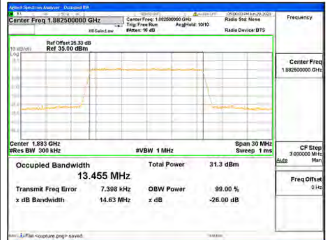
Band25 / 15MHz / QPSK/ Mid CH
