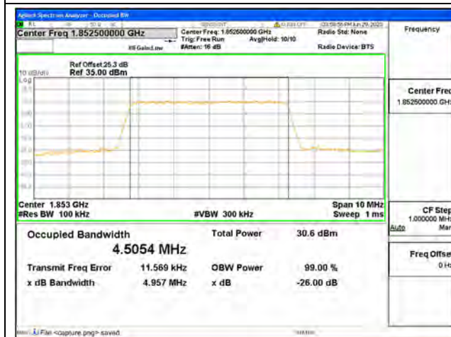
Band2 / 5MHz / 64QAM/ Low CH
