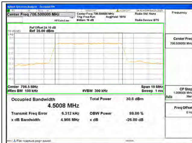
Band17 / 5MHz / QPSK/ Low CH
