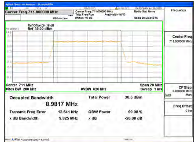
Band12 / 10MHz / QPSK/ High CH
