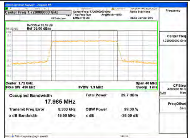
Band4 / 20MHz / 64QAM/ Low CH
