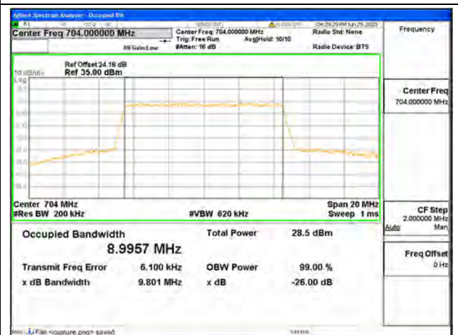
Band12 / 10MHz / 64QAM/ Low CH
