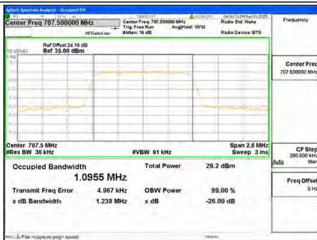
Band12 / 1.4MHz / 16QAM/ Mid CH
