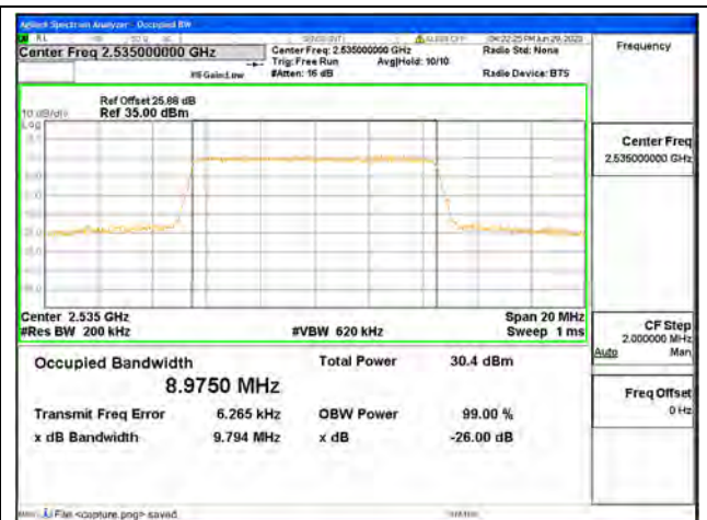
Band7 / 10MHz / 16QAM/ Mid CH
