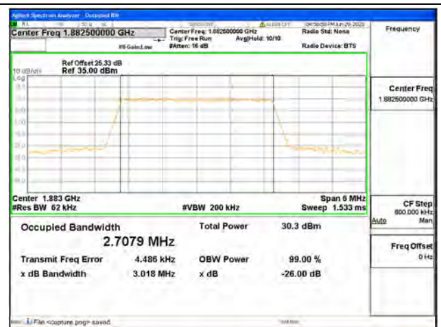
Band25 / 3MHz / 16QAM/ Mid CH
