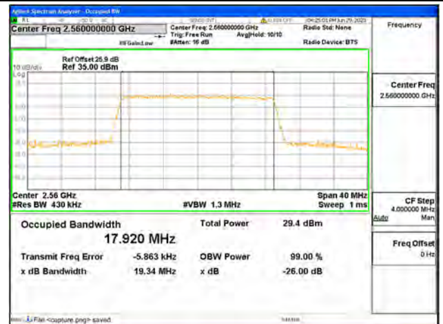
Band7 / 20MHz / 64QAM/ High CH
