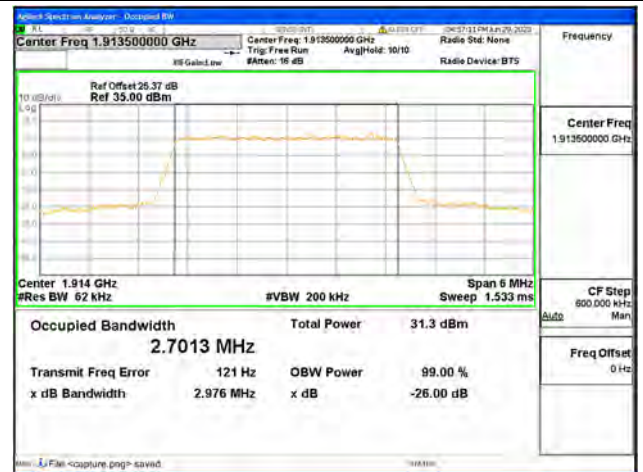
Band25 / 3MHz / QPSK/ High CH
