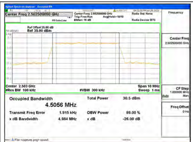
Band7 / 5MHz / 16QAM/ Low CH
