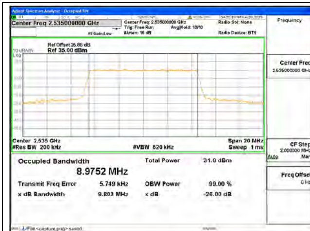
Band7 / 10MHz / QPSK/ Mid CH
