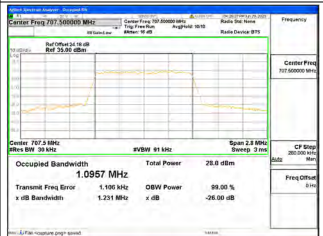
Band12 / 1.4MHz / 64QAM/ Mid CH
