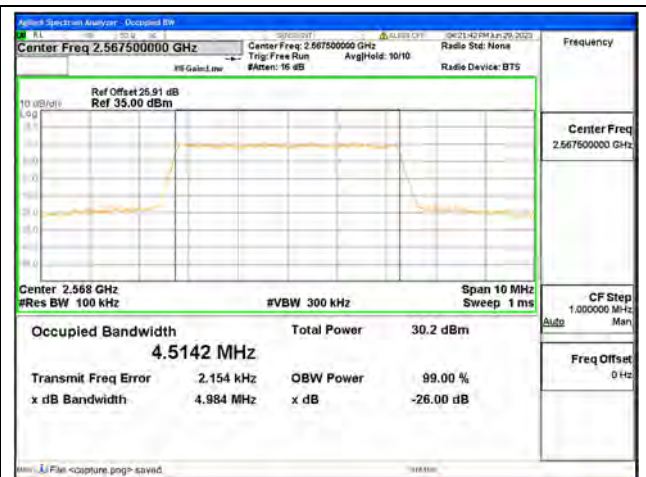
Band7 / 5MHz / 16QAM/ High CH
