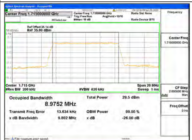
Band4 / 10MHz / 64QAM/ Low CH
