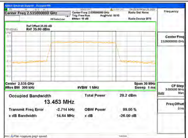
Band7 / 15MHz / 64QAM/ Mid CH
