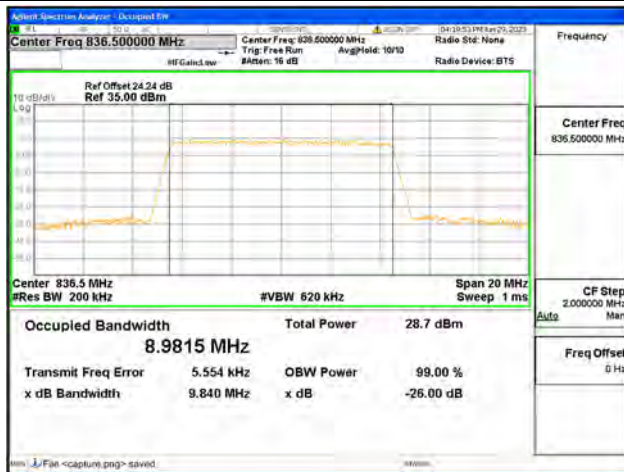
Band5 / 10MHz / 64QAM/ Mid CH
