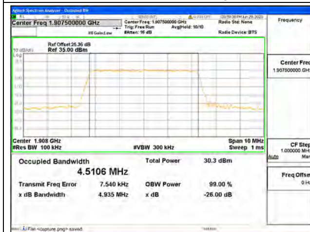
Band2 / 5MHz / 64QAM/ High CH
