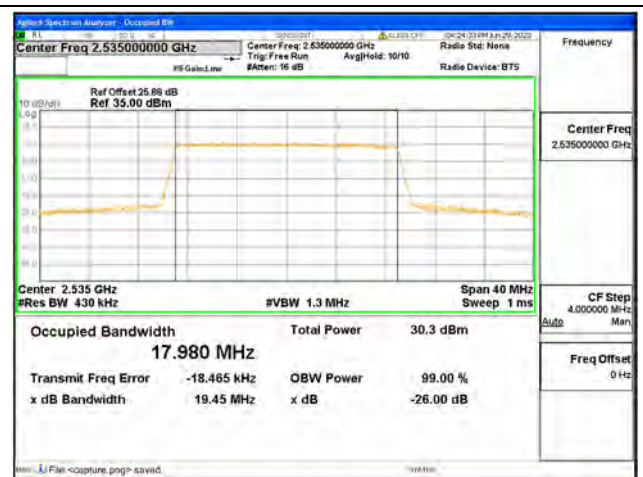
Band7 / 20MHz / 16QAM/ Mid CH
