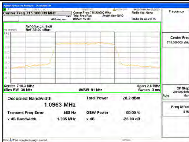
Band12 / 1.4MHz / 64QAM/ High CH
