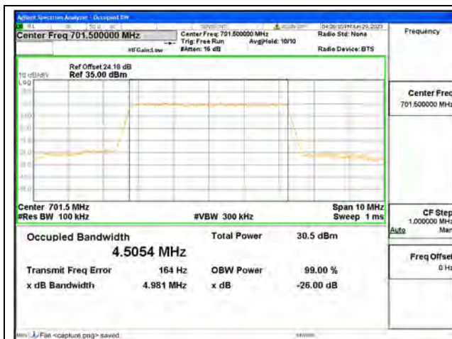
Band12 / 5MHz / QPSK/ Low CH
