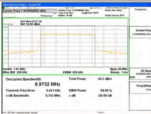
Band25 / 10MHz / 16QAM/ High CH
