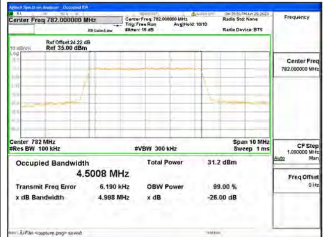
Band13 / 5MHz / QPSK/ Mid CH
