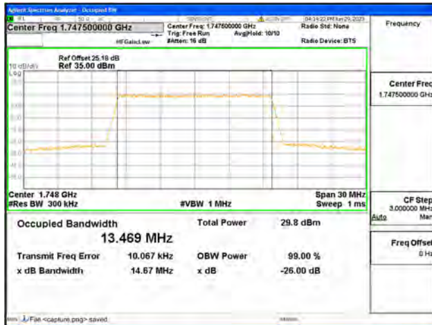
Band4 / 15MHz / 64QAM/ High CH
