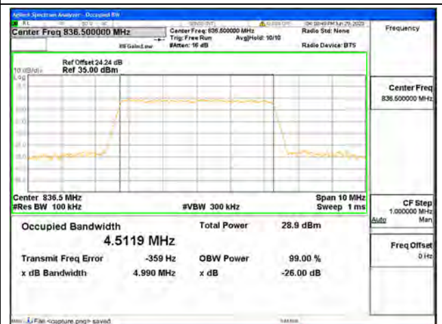
Band5 / 5MHz / 64QAM/ Mid CH
