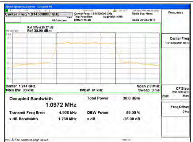
Band25 / 1.4MHz / 16QAM/ High CH
