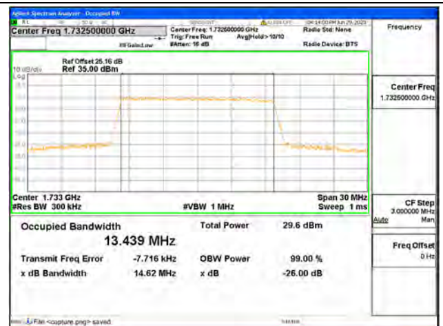
Band4 / 15MHz / 64QAM/ Mid CH
