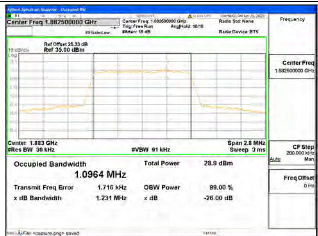
Band25 / 1.4MHz / 64QAM/ Mid CH
