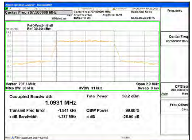
Band12 / 1.4MHz / QPSK/ Mid CH
