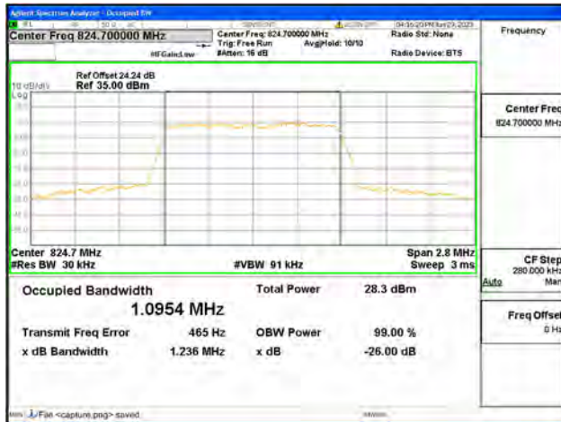
Band5 / 1.4MHz / 64QAM/ Low CH
