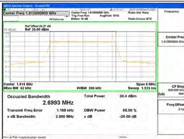
Band25 / 3MHz / 16QAM/ High CH
