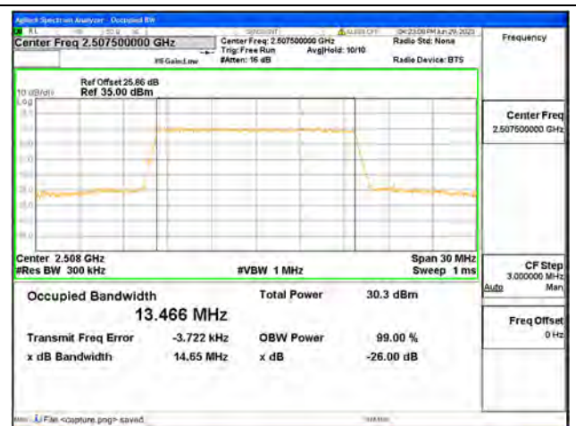
Band7 / 15MHz / 16QAM/ Low CH
