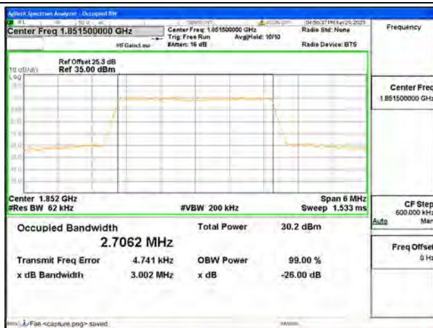
Band25 / 3MHz / 16QAM/ Low CH
