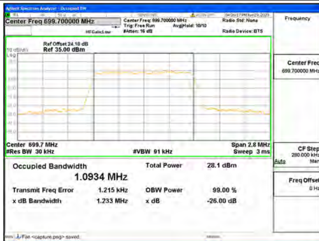
Band12 / 1.4MHz / 64QAM/ Low CH
