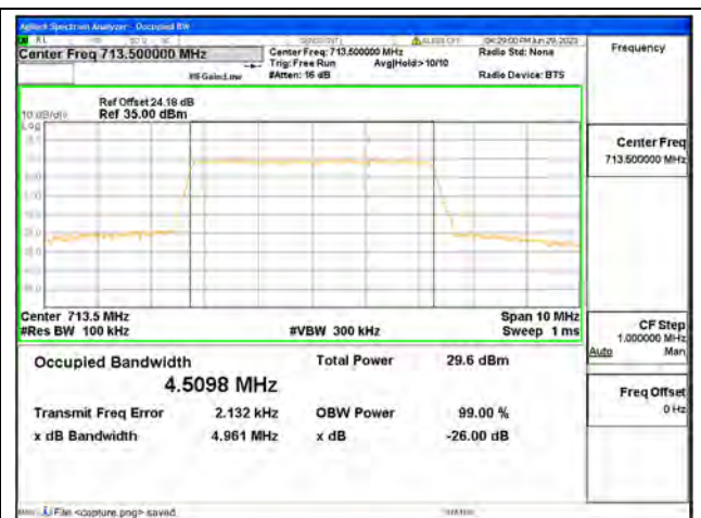
Band12 / 5MHz / 16QAM/ High CH
