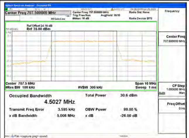
Band12 / 5MHz / QPSK/ Mid CH
