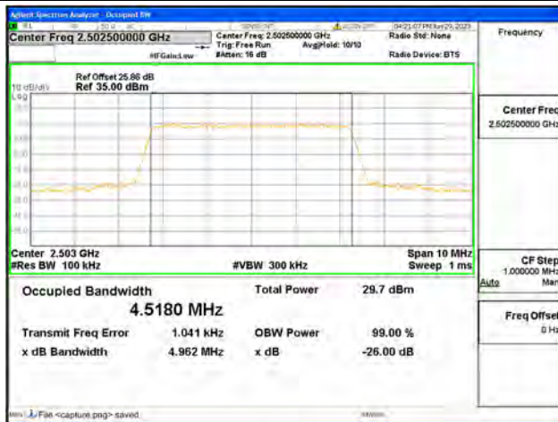
Band7 / 5MHz / 64QAM/ Low CH
