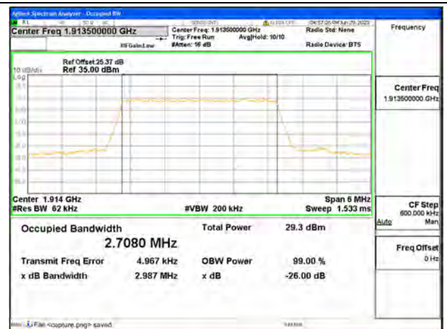
Band25 / 3MHz / 64QAM/ High CH
