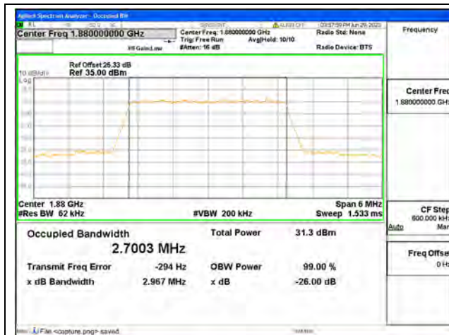
Band2 / 3MHz / QPSK/ Mid CH
