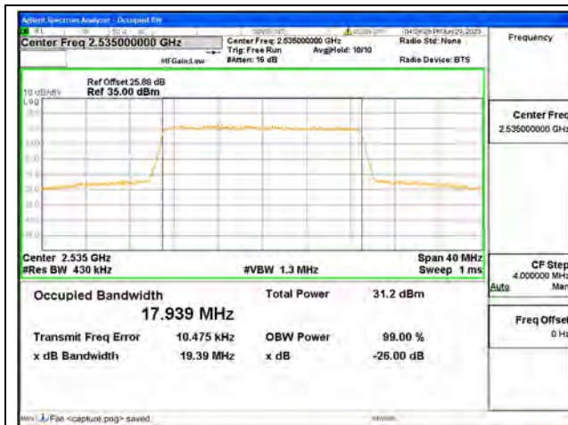
Band7 / 20MHz / QPSK/ Mid CH
