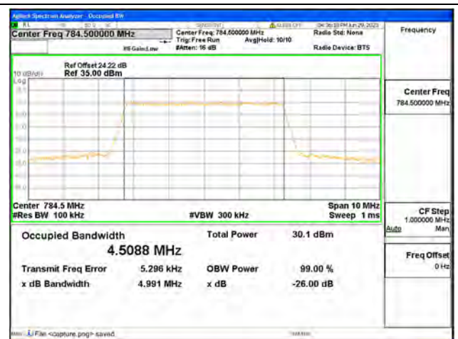
Band13 / 5MHz / 16QAM/ High CH
