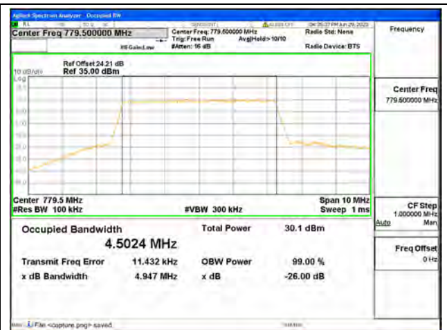
Band13 / 5MHz / 16QAM/ Low CH
