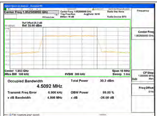
Band25 / 5MHz / 16QAM/ Low CH
