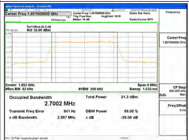
Band2 / 3MHz / QPSK/ Low CH
