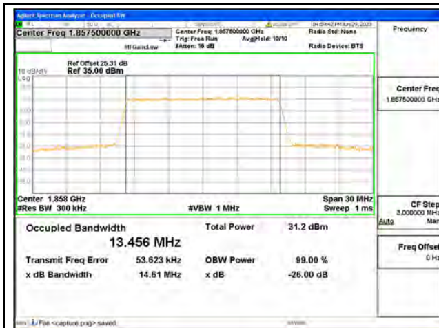
Band25 / 15MHz / QPSK/ Low CH
