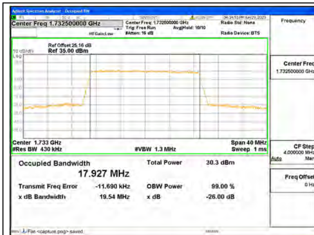
Band4 / 20MHz / QPSK/ Mid CH
