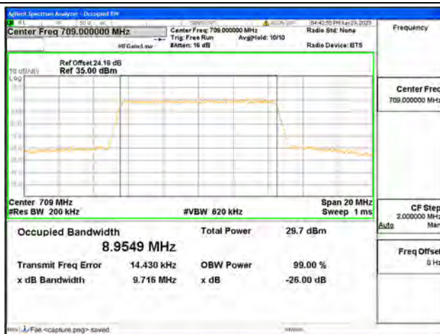
Band17 / 10MHz / 16QAM/ Low CH
