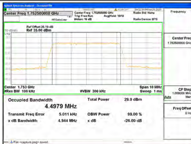
Band4 / 5MHz / 64QAM/ High CH
