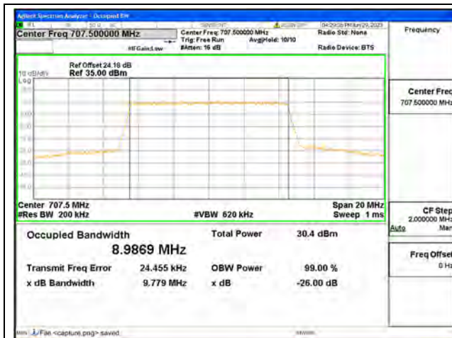
Band12 / 10MHz / QPSK/ Mid CH
