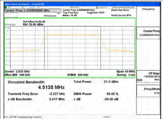
Band7 / 5MHz / QPSK/ Mid CH
