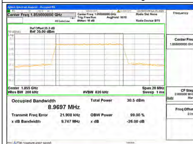
Band2 / 10MHz / 16QAM/ Low CH
