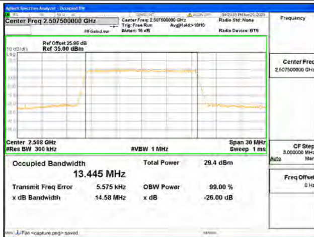
Band7 / 15MHz / 64QAM/ Low CH
