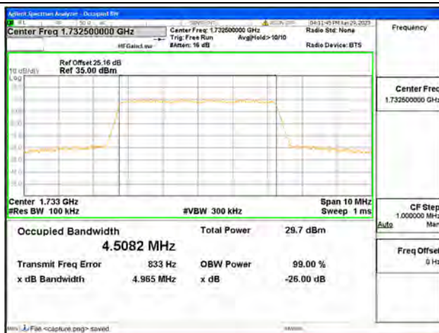
Band4 / 5MHz / 16QAM/ Mid CH
