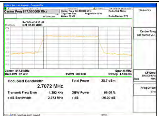
Band5 / 3MHz / 64QAM/ High CH
