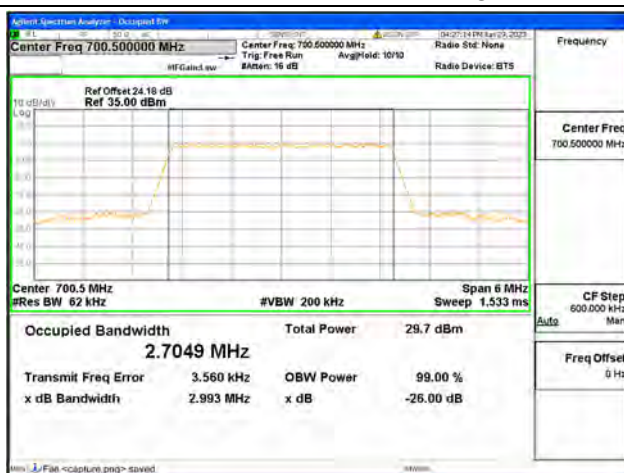
Band12 / 3MHz / 16QAM/ Low CH
